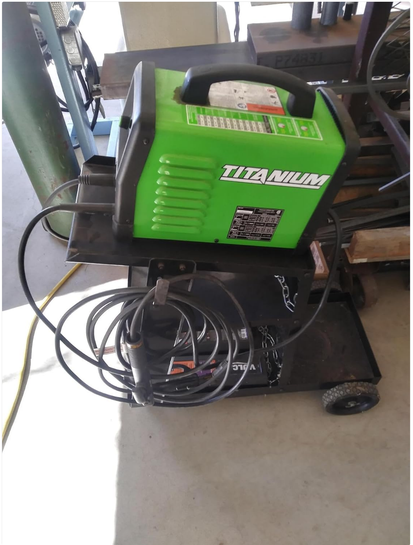
Figure 3.1: Titanium Stick 225 Inverter Welder on a welding cart, showcasing its compact size and portability.
