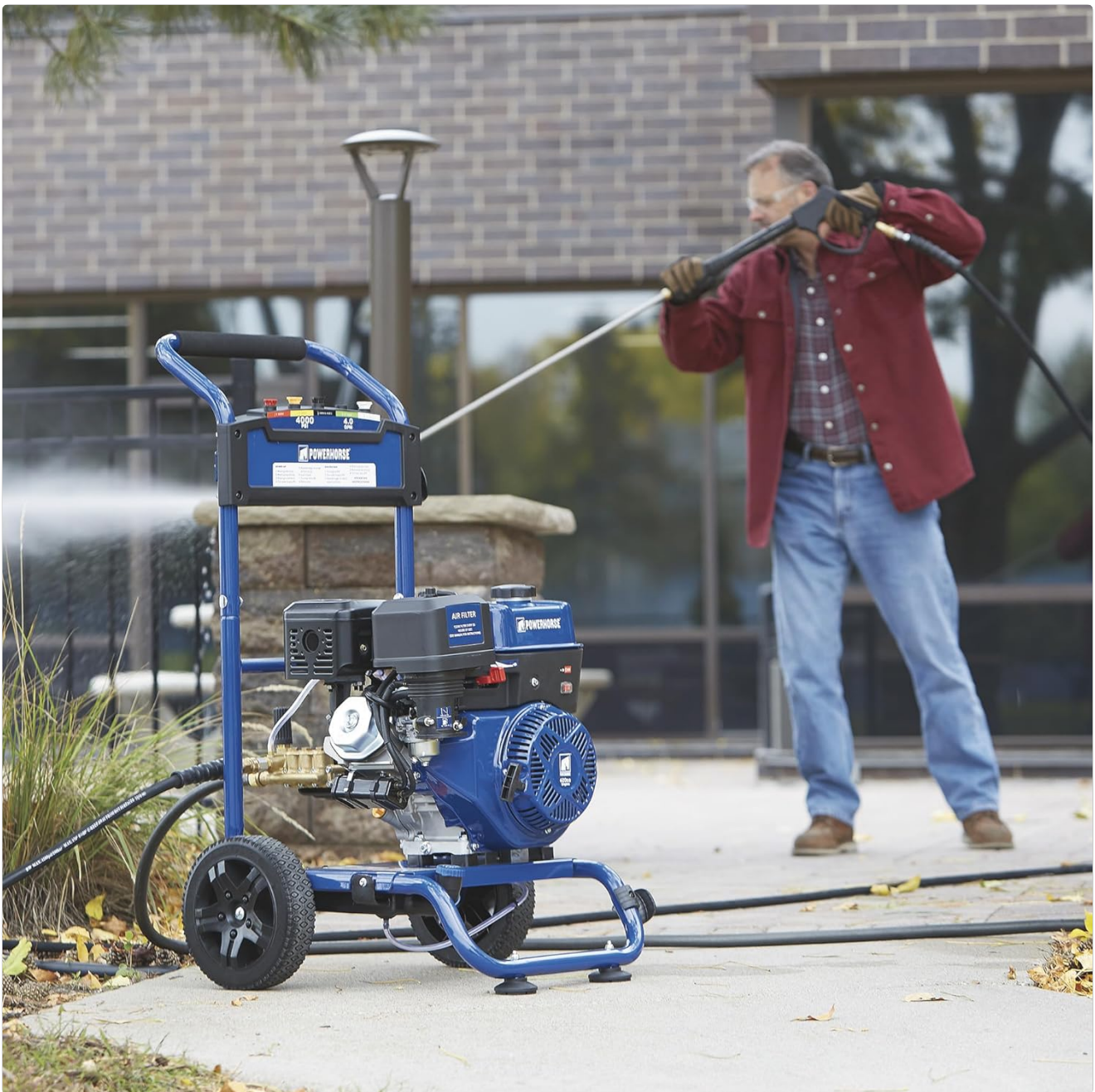
Figure 5: Operating the pressure washer to clean a patio surface.
