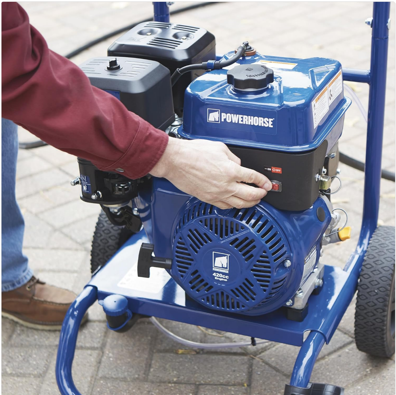
Figure 4: Turning the engine switch to the 'ON' position.
