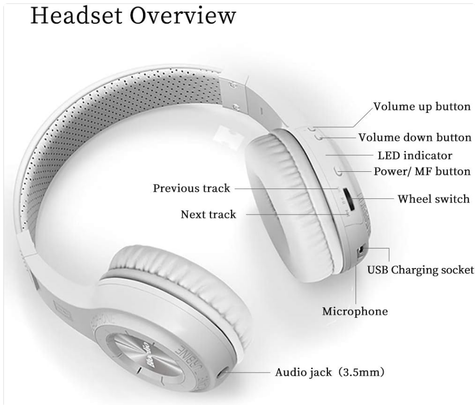
Figure 1: Headset Overview with labeled components.
