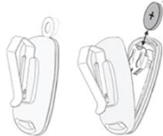
Image: A diagram illustrating the steps for replacing the battery in the remote control.
