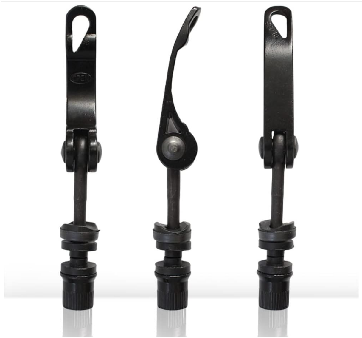
Figure 4: Different positions of the quick release lever, illustrating open and closed states.
