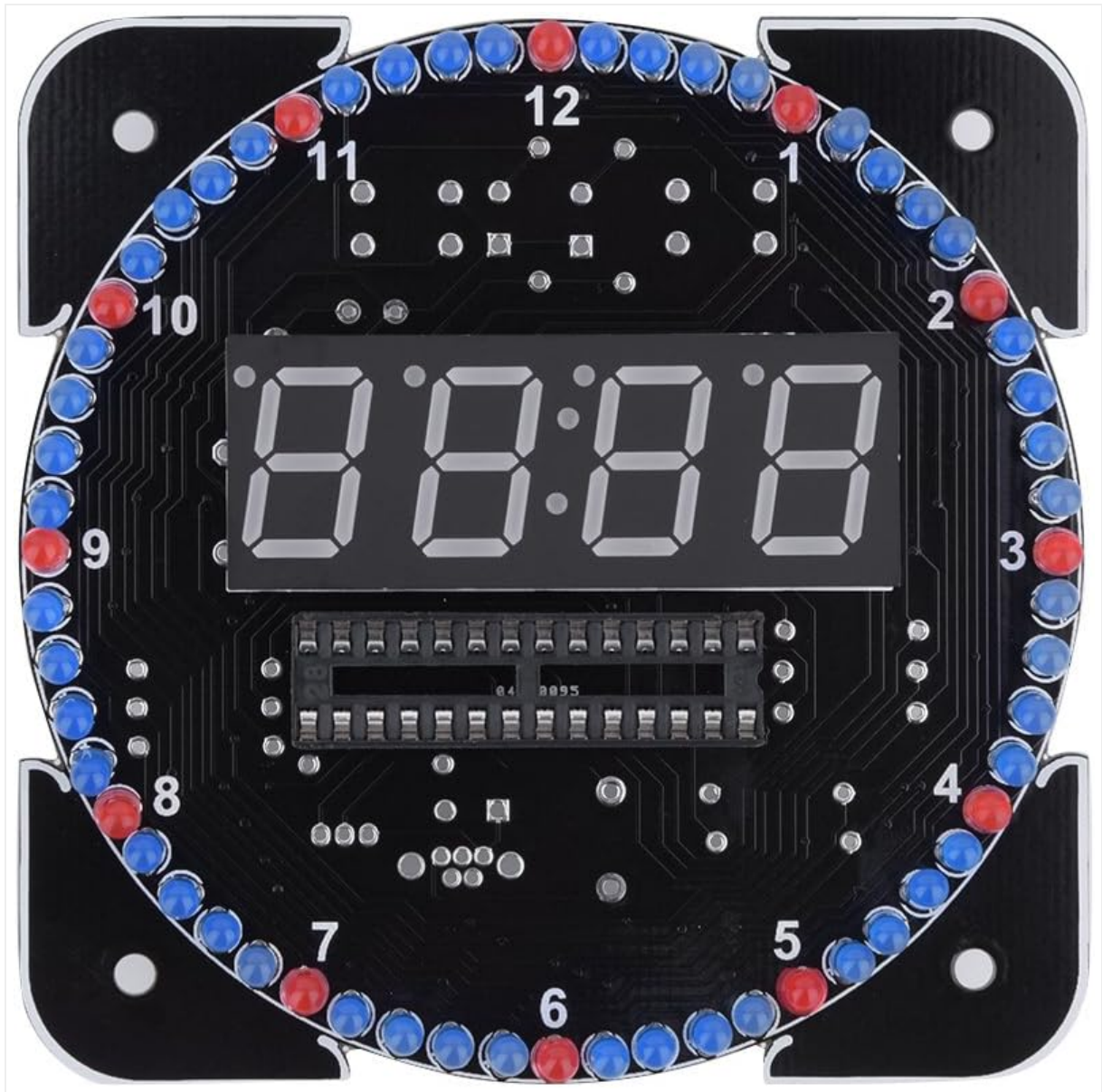
Image 4.1: The fully assembled Printed Circuit Board (PCB) of the digital alarm clock, showing the central 4-digit display and the surrounding red and blue LEDs.
