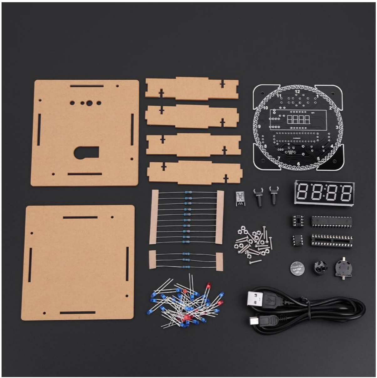
Image 3.1: All components of the DIY Digital Alarm Clock Kit, including the PCB, digital display, various electronic parts, and a USB cable, laid out on a flat surface.
