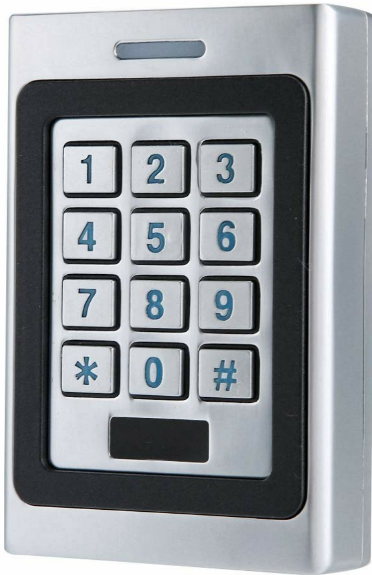
Figure 1.1: Front view of the Sonew A7-RK-EM RFID Access Controller. This image shows the silver-colored unit with a black keypad featuring numerical buttons (0-9), asterisk (*), and hash (#) keys.
