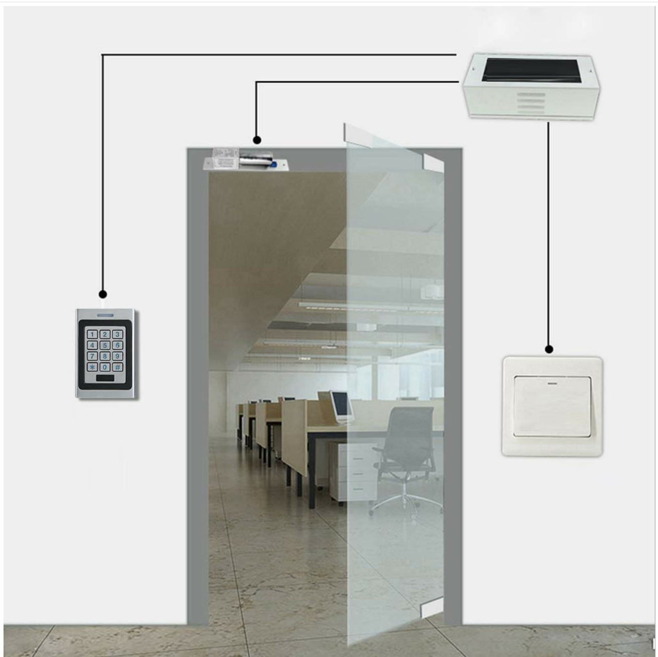
Figure 5.2: Illustrative wiring diagram showing the connection of the access controller to a door lock, power supply, and exit button.
