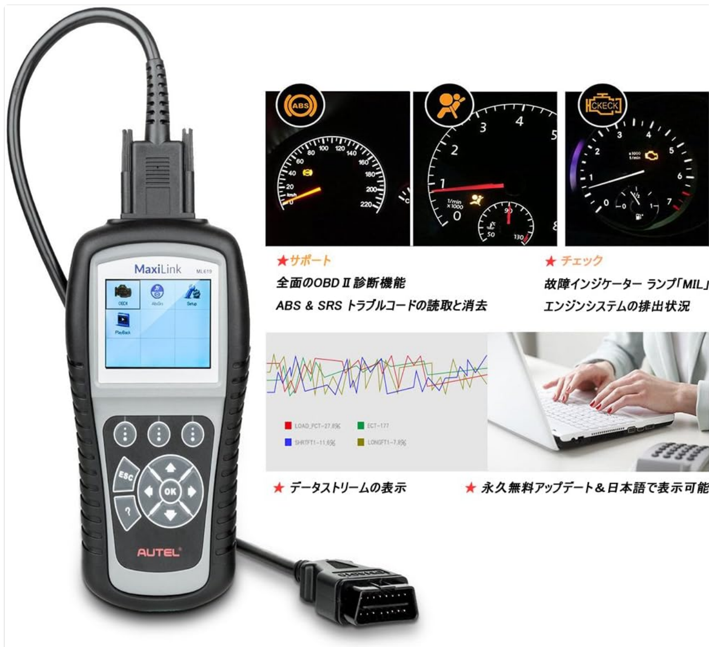
Figure 7.1: Autel ML619 showing data stream and diagnostic indicators, with an illustration of data printing to a laptop.
