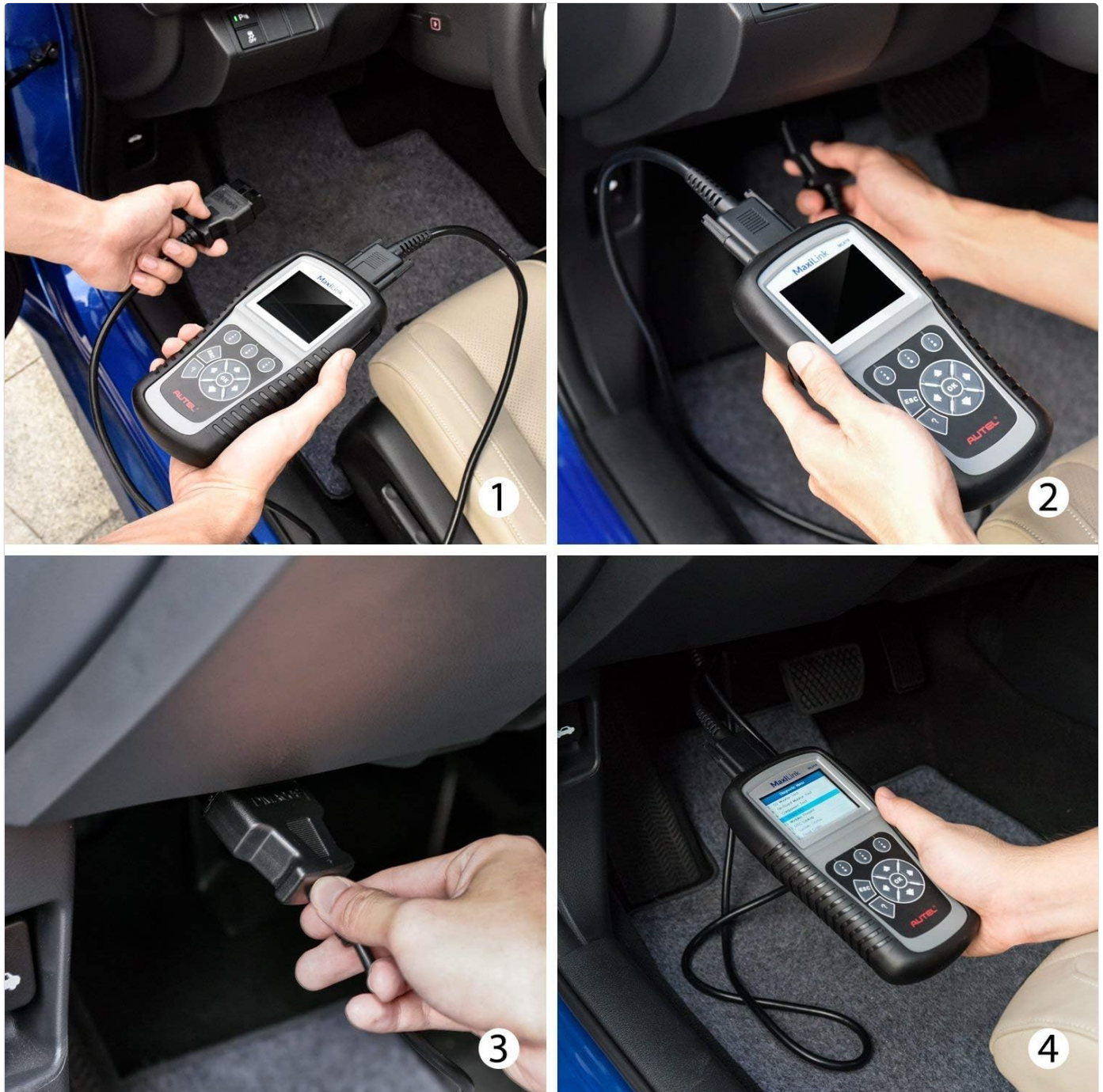
Figure 5.1: Step-by-step connection process for the Autel ML619 to a vehicle's OBD2 port.
