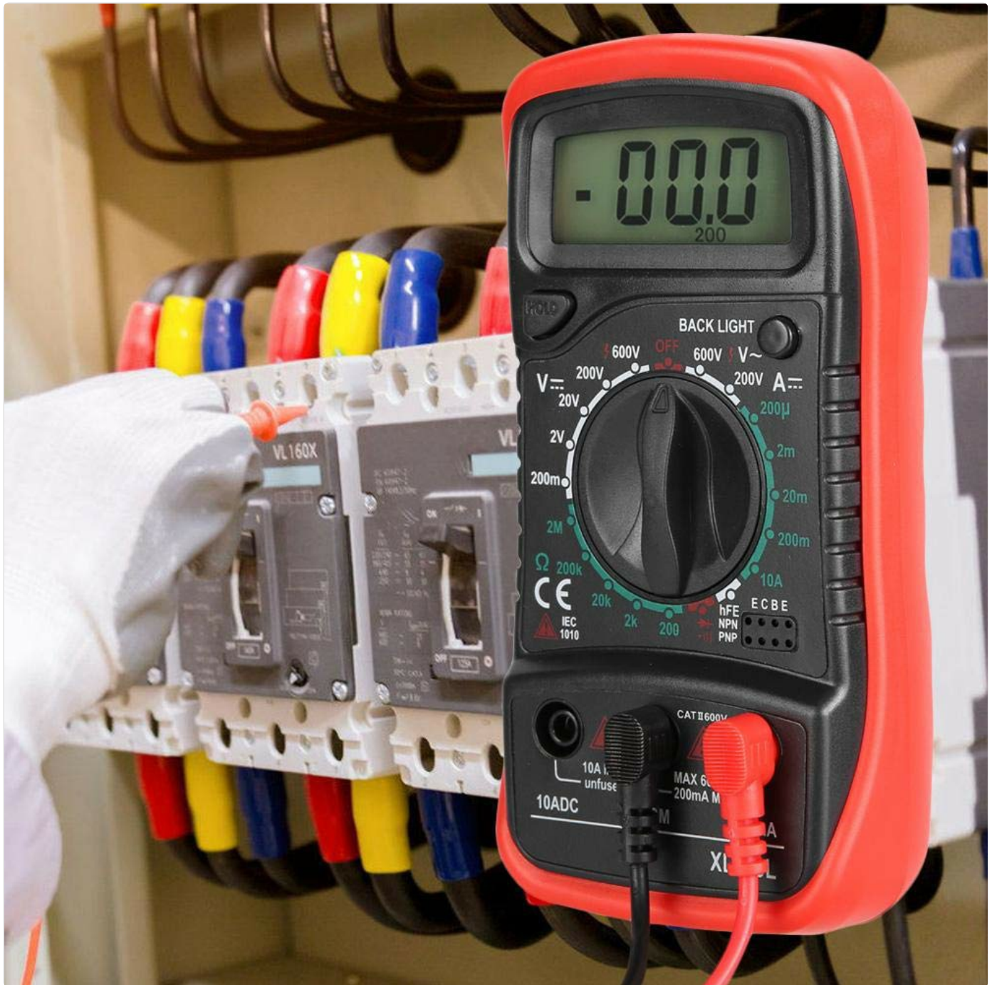
Figure 4: Example of using the multimeter to measure voltage in an electrical panel.
