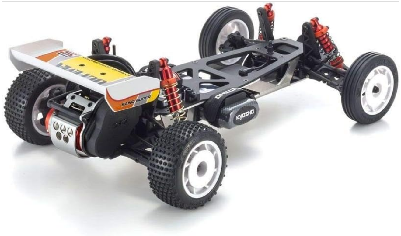
Figure 4.2: Top-down view of the Kyosho Ultima chassis, highlighting the layout of the internal components and the glass-reinforced upper deck.
