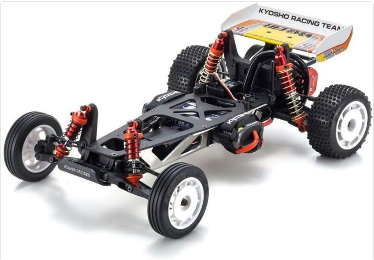
Figure 4.1: View of the Kyosho Ultima chassis from the side, showing the monocoque aluminum frame and internal components.
