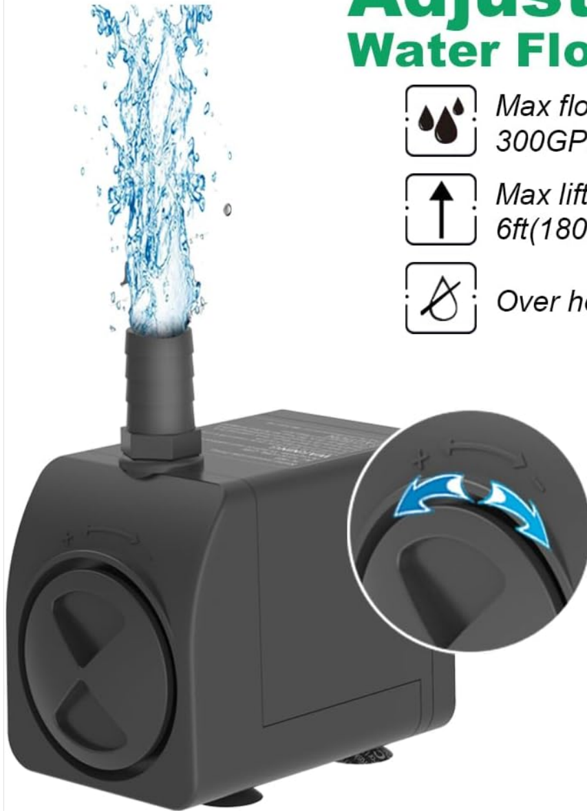
Image 2.2: Adjustable Water Flow Rate. This image illustrates the pump's adjustable flow knob, showing a maximum flow rate of 300 GPH (1100 L/h) and a maximum lift height of 6 ft (180 cm), along with overheating protection.
