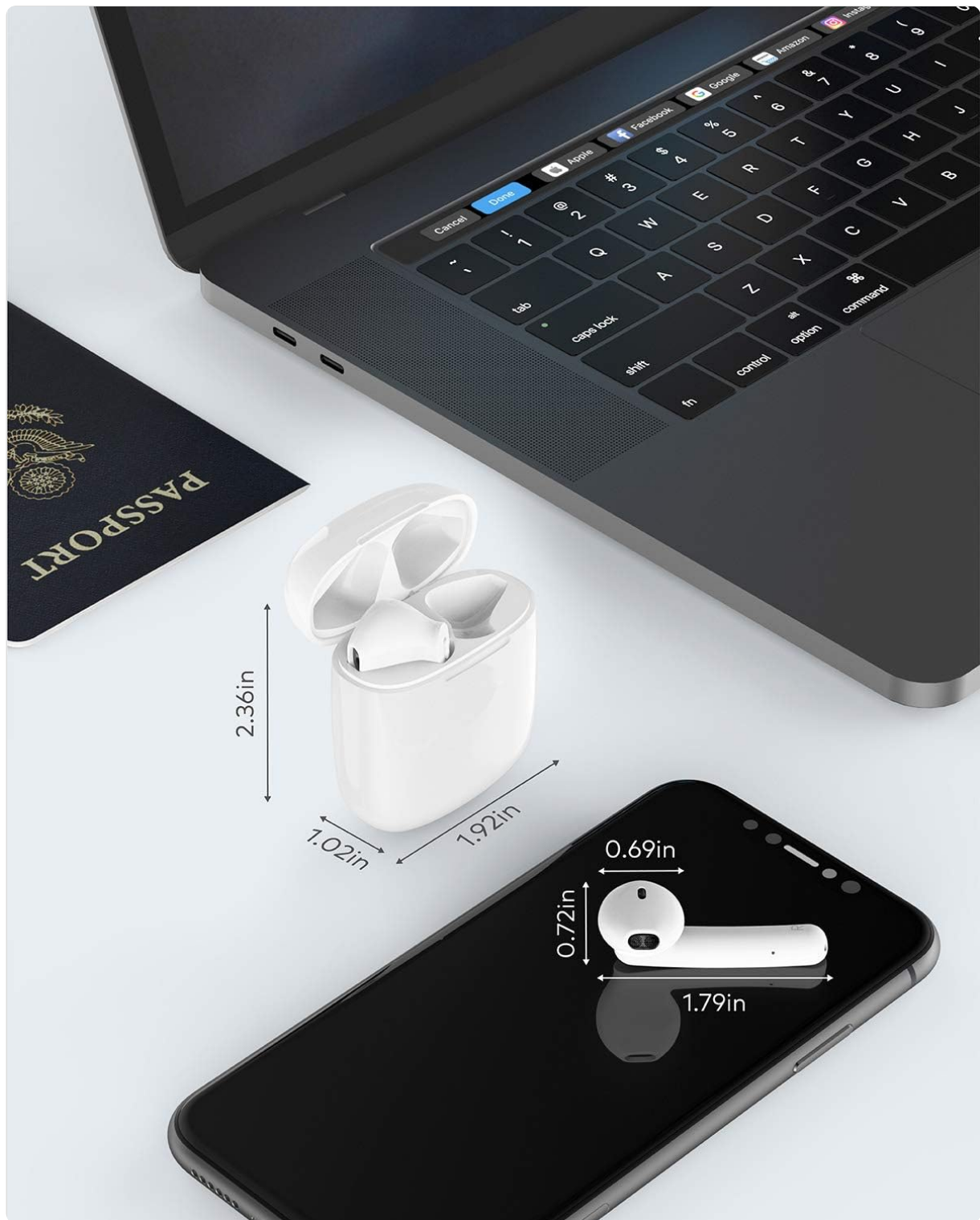
Figure 4.2: Dimensions of the BEBEN T12 earbuds and charging case.
