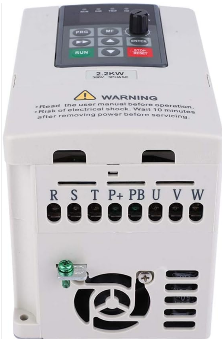
Figure 5.3: Rear view of the VFD, clearly showing the input (R, S, T) and output (U, V, W) terminals, plus braking resistor terminals (P+, PB).
