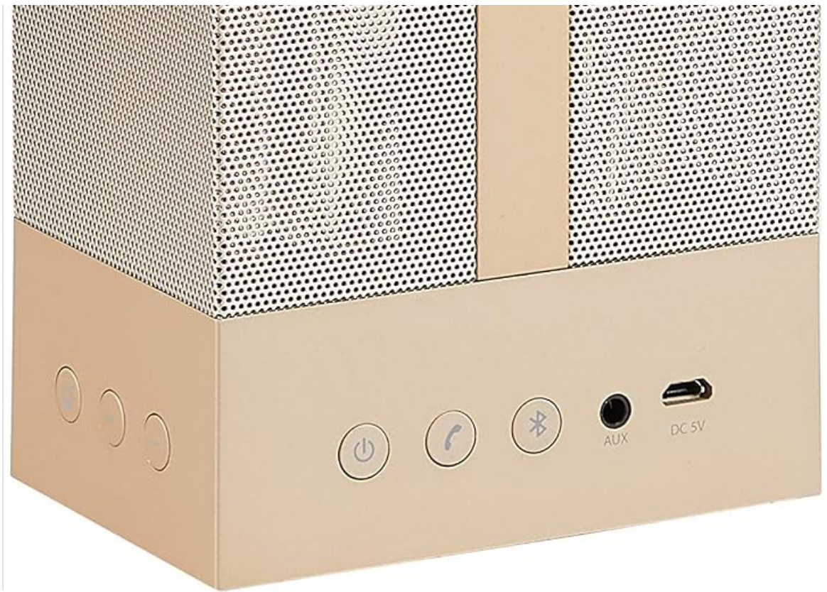
Figure 2: Rear view of the speaker, highlighting the DC 5V charging port and AUX input.
