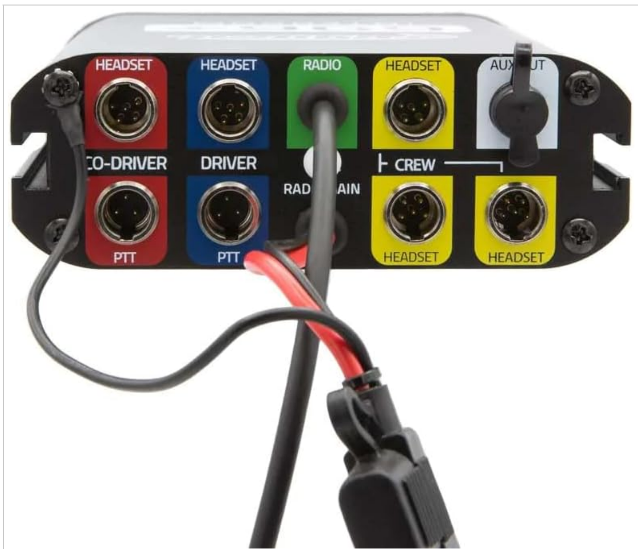
Rear view of the RRP696 Plus Intercom, illustrating the various ports for driver, co-driver, radio, and crew headsets, along with PTT and auxiliary output connections.
