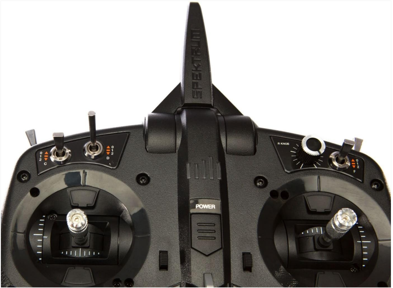
Figure 2: Top view of the Spektrum DX8e 8-Channel DSMX Transmitter, highlighting the various switches and trim controls.
