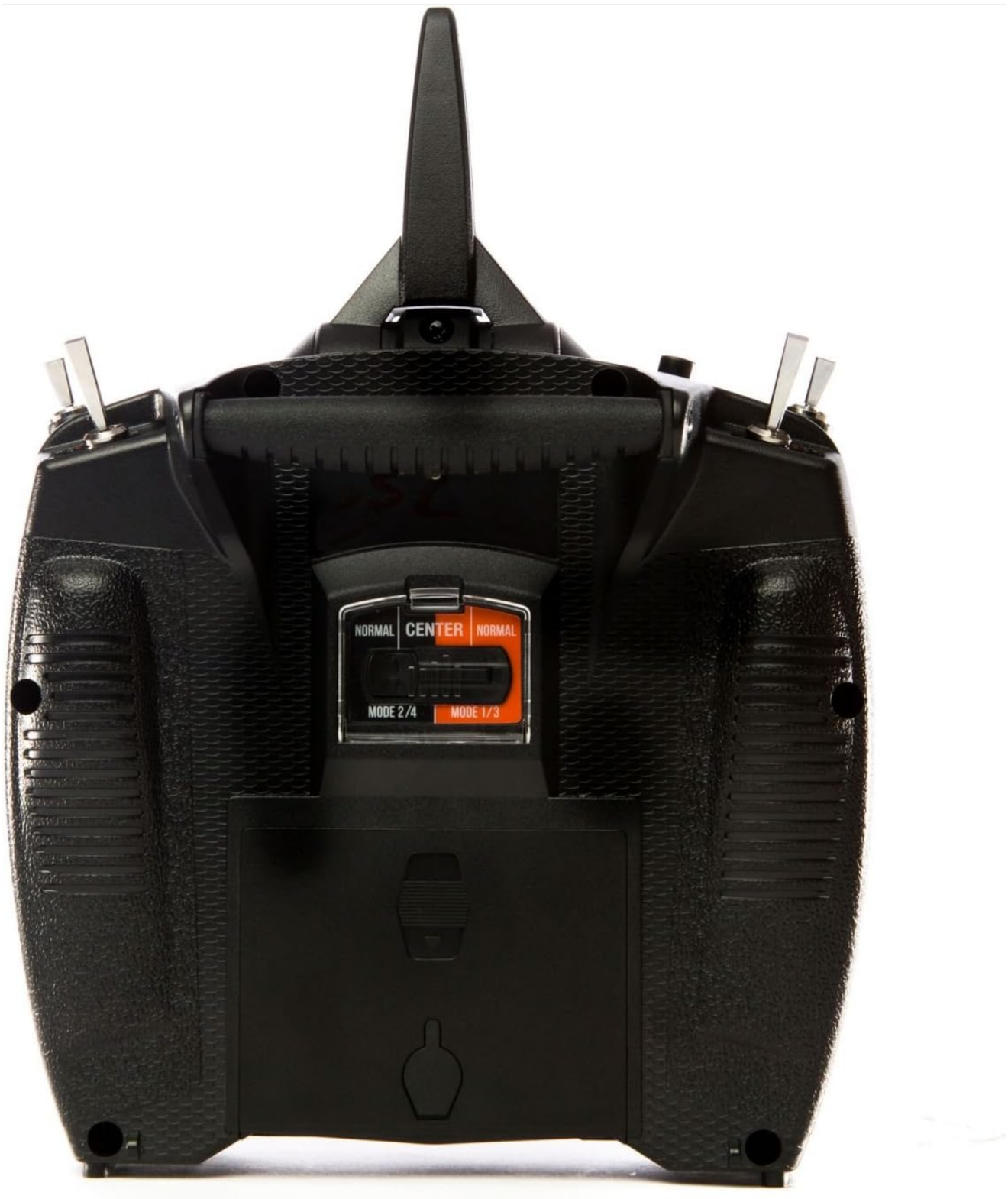
Figure 3: Rear view of the Spektrum DX8e 8-Channel DSMX Transmitter, showing the battery cover and the mode selection switch.
