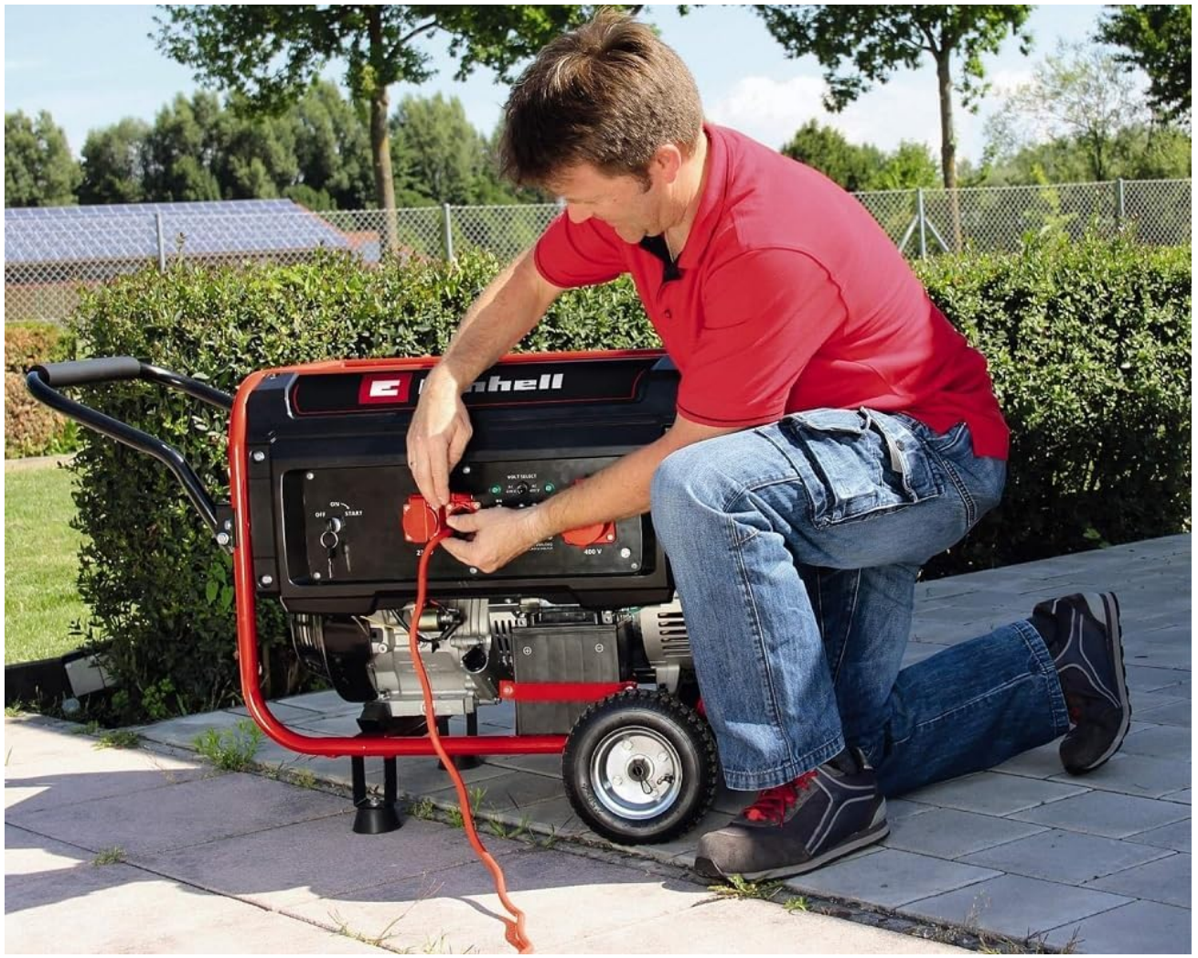
Image: A person connecting an electrical cord to one of the 230 V sockets on the generator's control panel.
