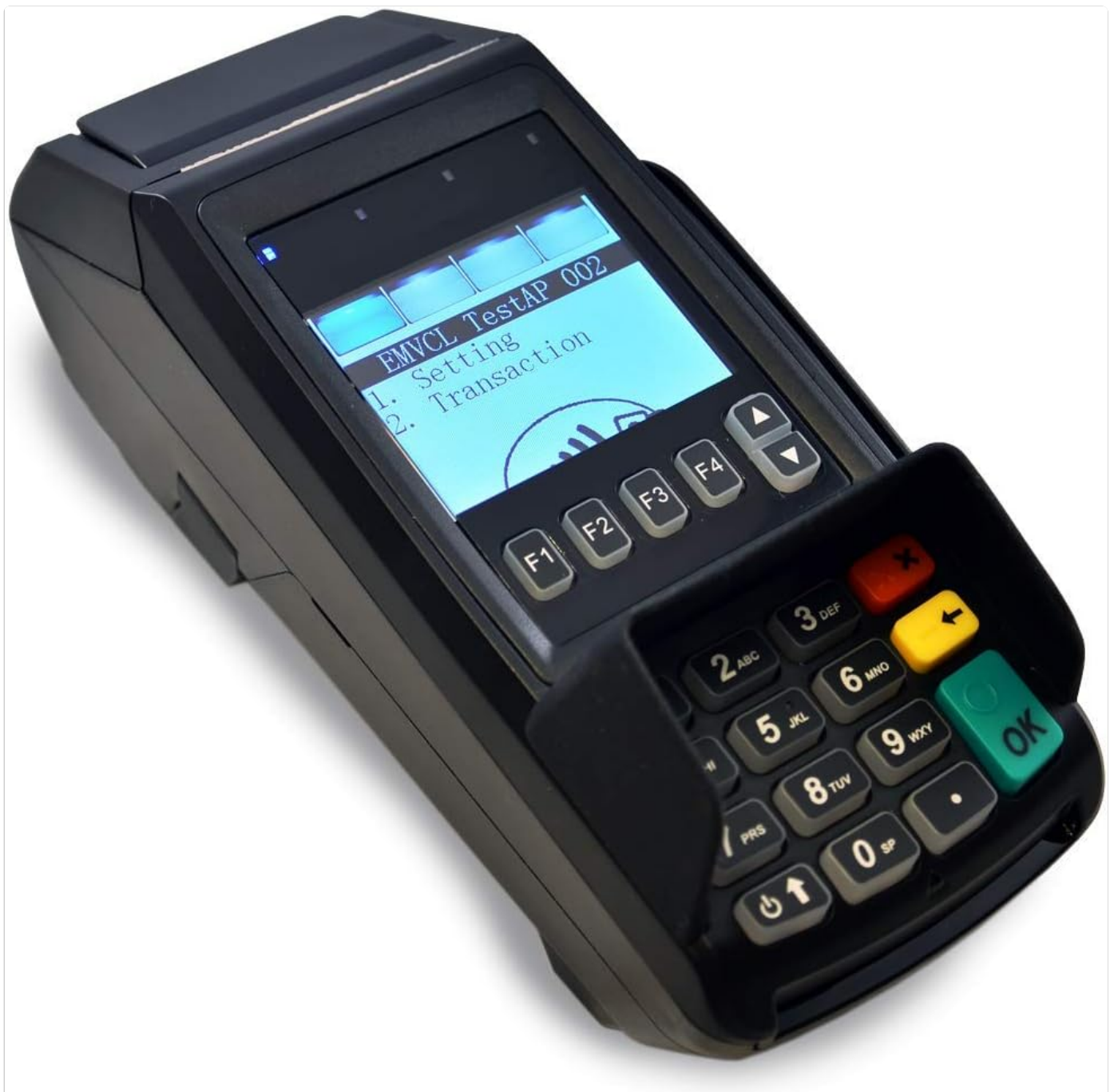
Figure 1: Dejavoo Z8 Terminal showing the main display and keypad. The screen indicates options for 'Setting' and 'Transaction'.
