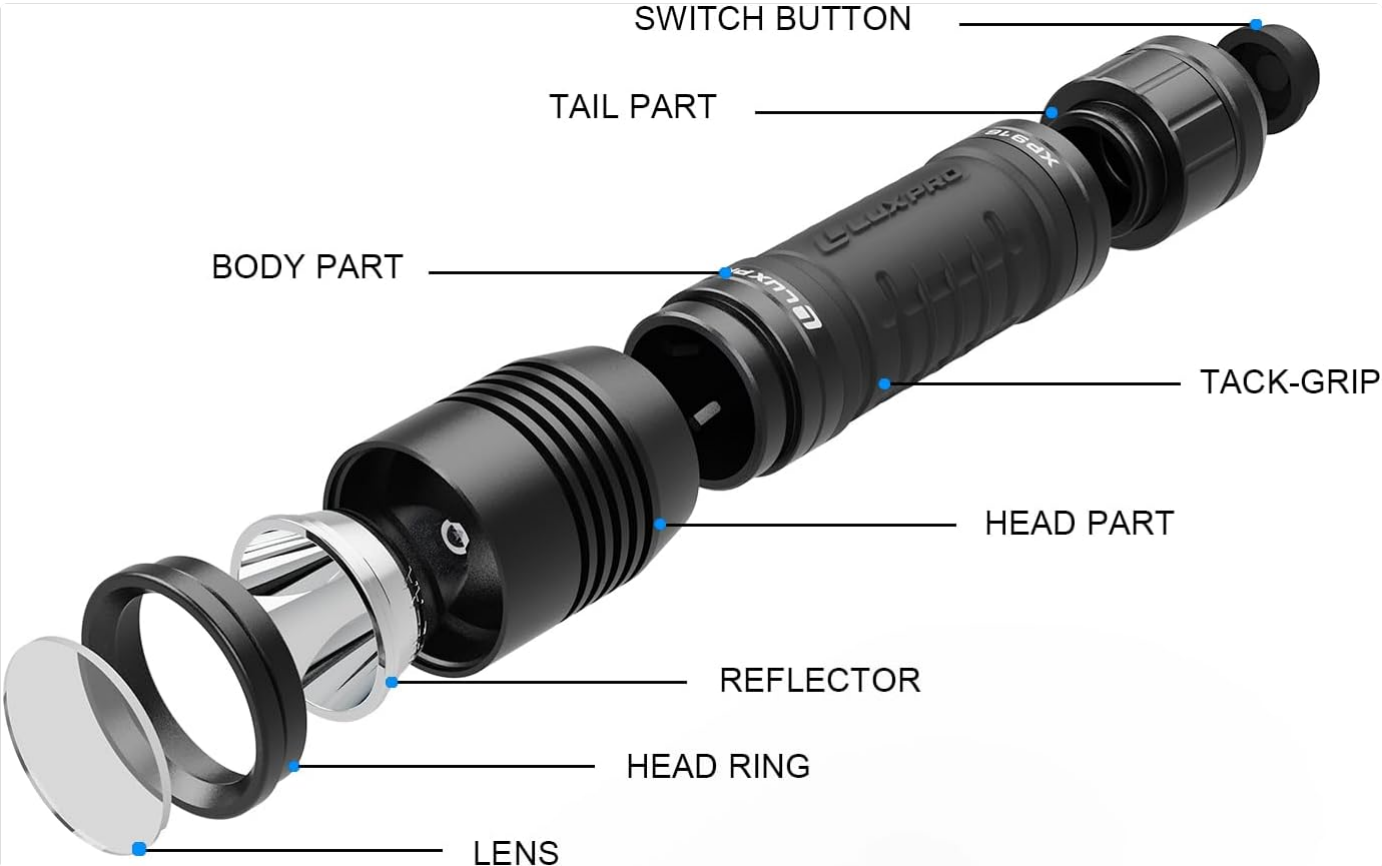
Figure 5: Exploded View of Flashlight Components. This diagram illustrates the internal and external parts of the flashlight, including the lens, reflector, head part, body part, TackGrip, tail part, and switch button, aiding in understanding its construction.
