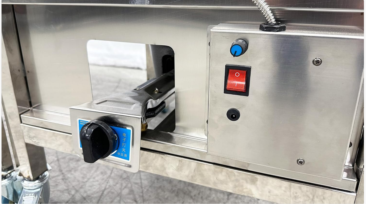
Image: Close-up view of the control panel, showing the propane control knob and the electric stirrer switch.
