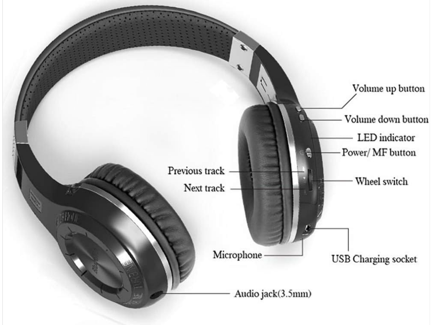
Figure 1: Headset Overview. This diagram highlights key features such as the Volume Up/Down buttons, LED indicator, Power/MF button, Wheel switch, Previous/Next track buttons, Microphone, USB Charging socket, and Audio jack (3.5mm).
