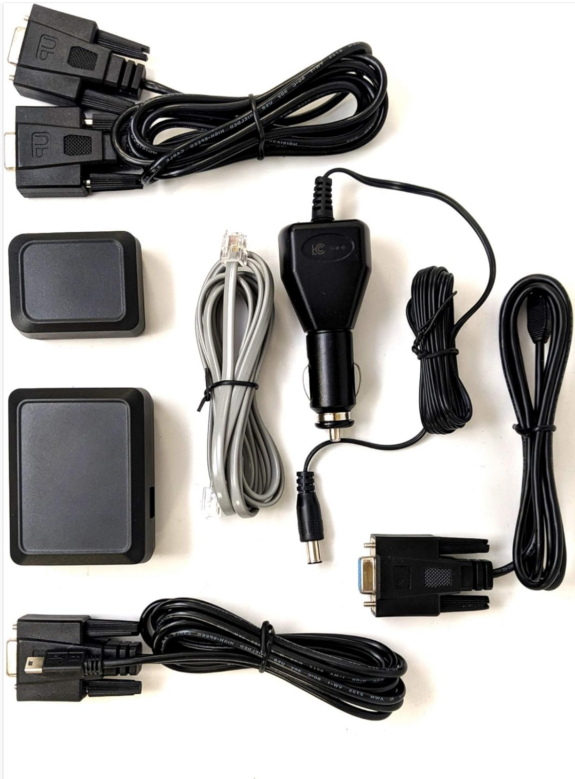
An overhead view of the Uniden BC-SGPS Universal Receiver Module Kit components, including the main GPS module, converter unit, various connection cables (RJ14, RS232, USB adapter), and a cigarette lighter power adapter, all neatly arranged.
