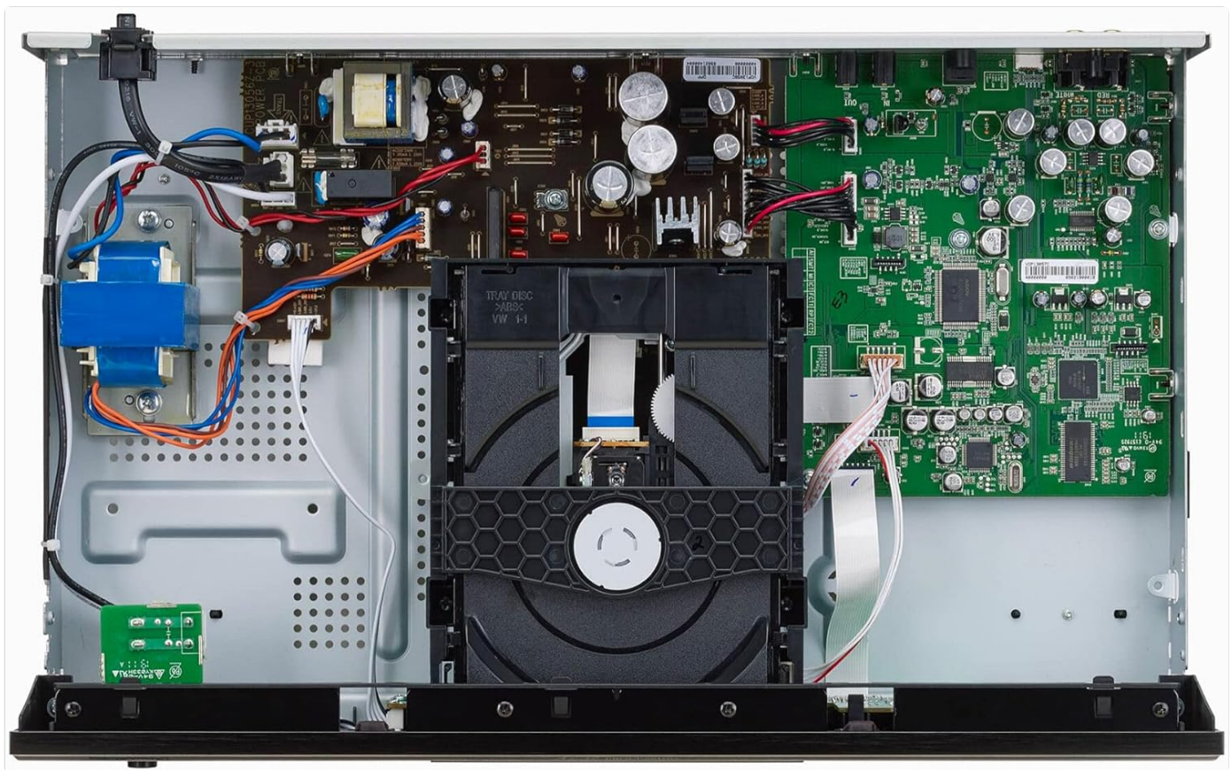
Figure 5: Internal components of the DCD-600NE, highlighting its robust construction for vibration resistance.
