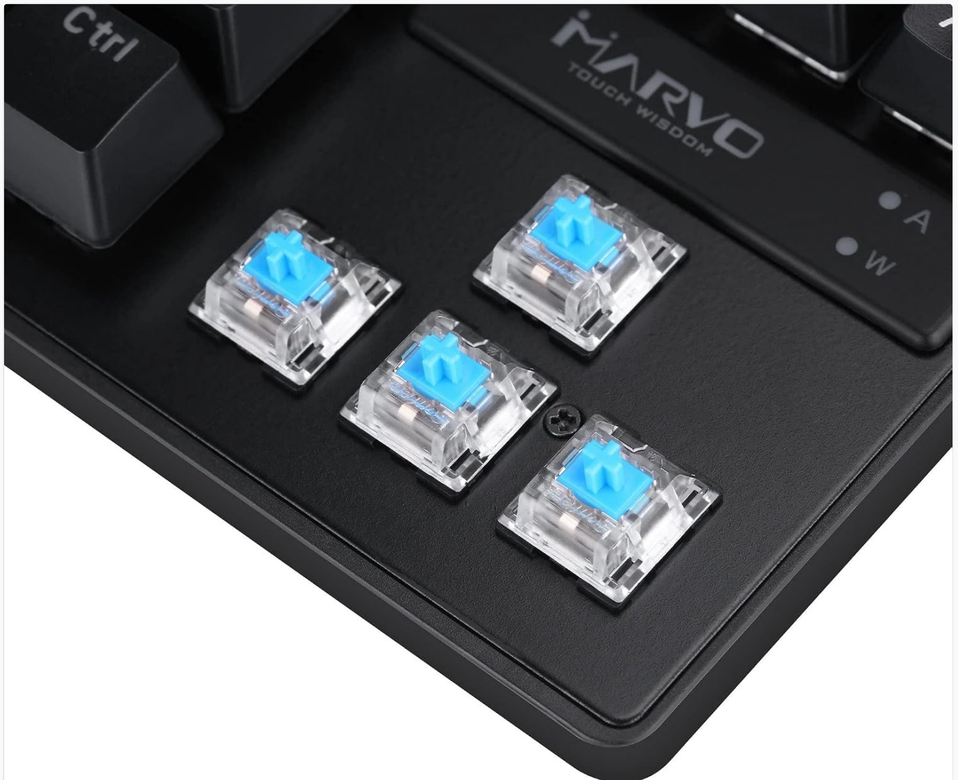
Image: A close-up view of the blue mechanical switches used in the MARVO KG901 keyboard, known for their tactile and clicky feedback.
