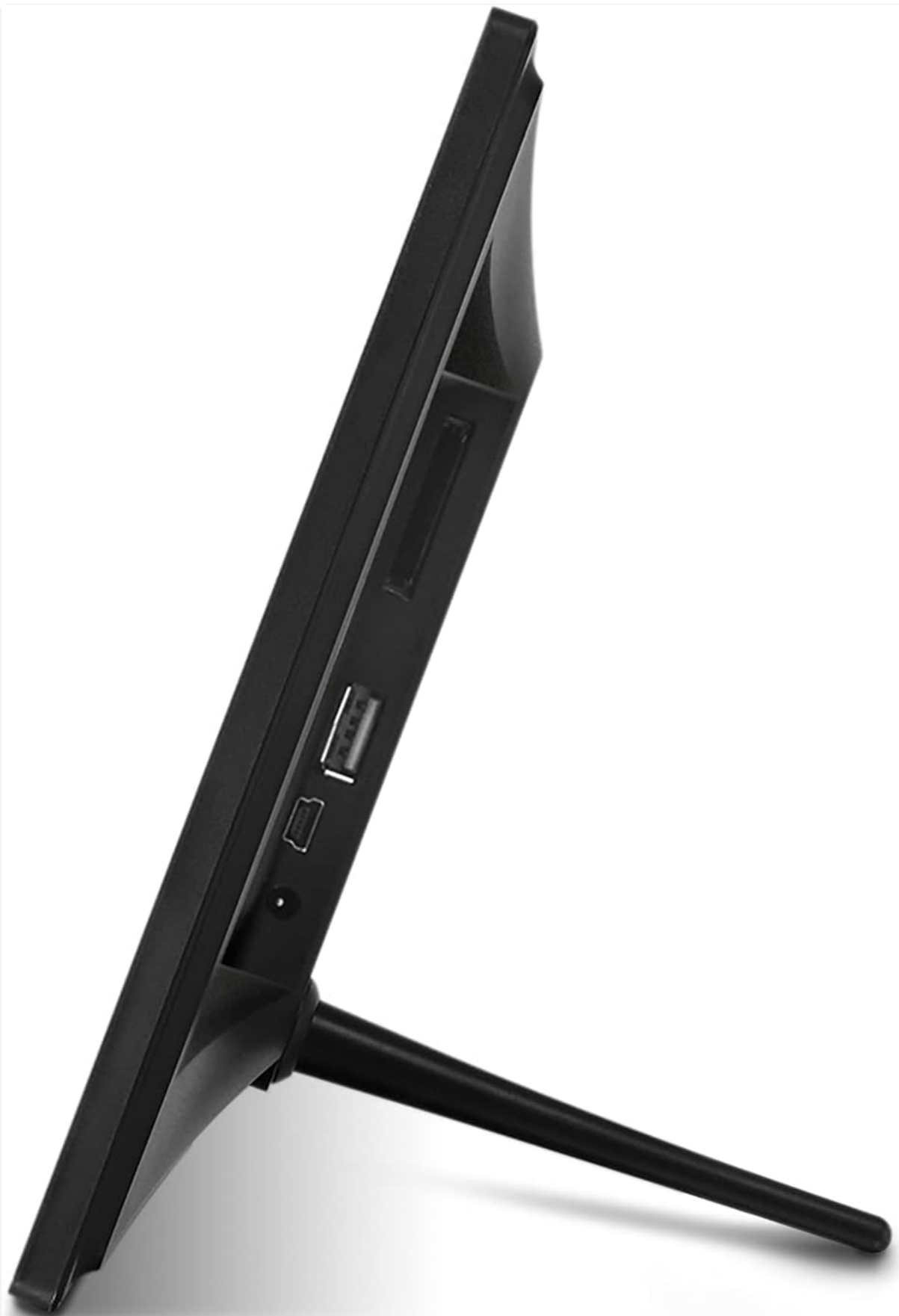
Image: A side profile of the digital photo frame, highlighting the various input ports. Visible ports include a full-size USB port, a micro-USB port, and an SD/SDHC card slot.
