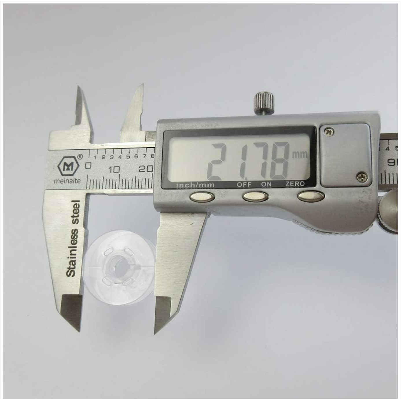
Figure 2: Bobbin diameter measurement, approximately 21.78 mm.
