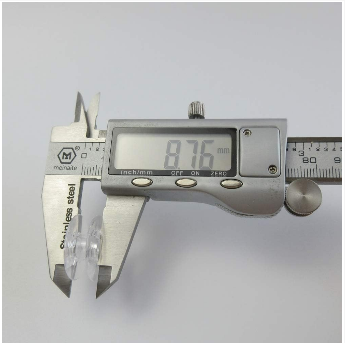
Figure 3: Bobbin height measurement, approximately 8.76 mm.
