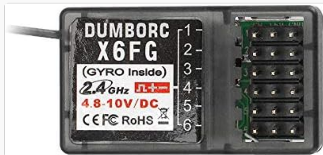
Figure 2: Front view of the DUMBORC X6FG receiver, showing the model name, 2.4GHz frequency, and power requirements (4.8-10V/DC).
