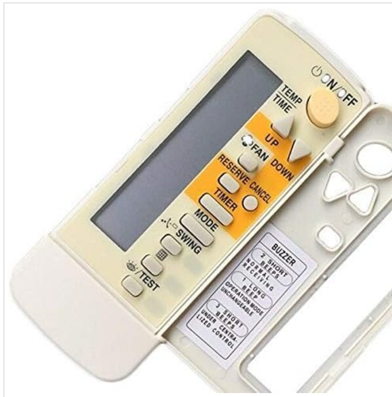
Figure 2: Remote controller with the sliding cover open, showing advanced function buttons and internal labels.
