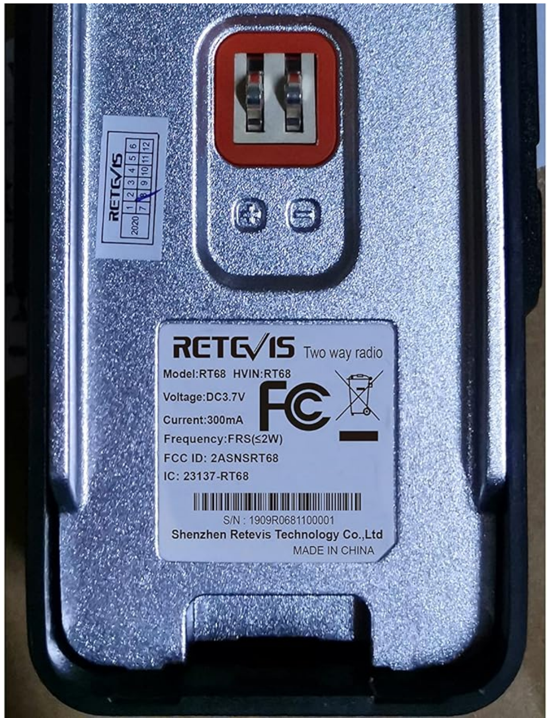
The back of the Retevis RT68 radio displays its model and FCC ID for compliance.
