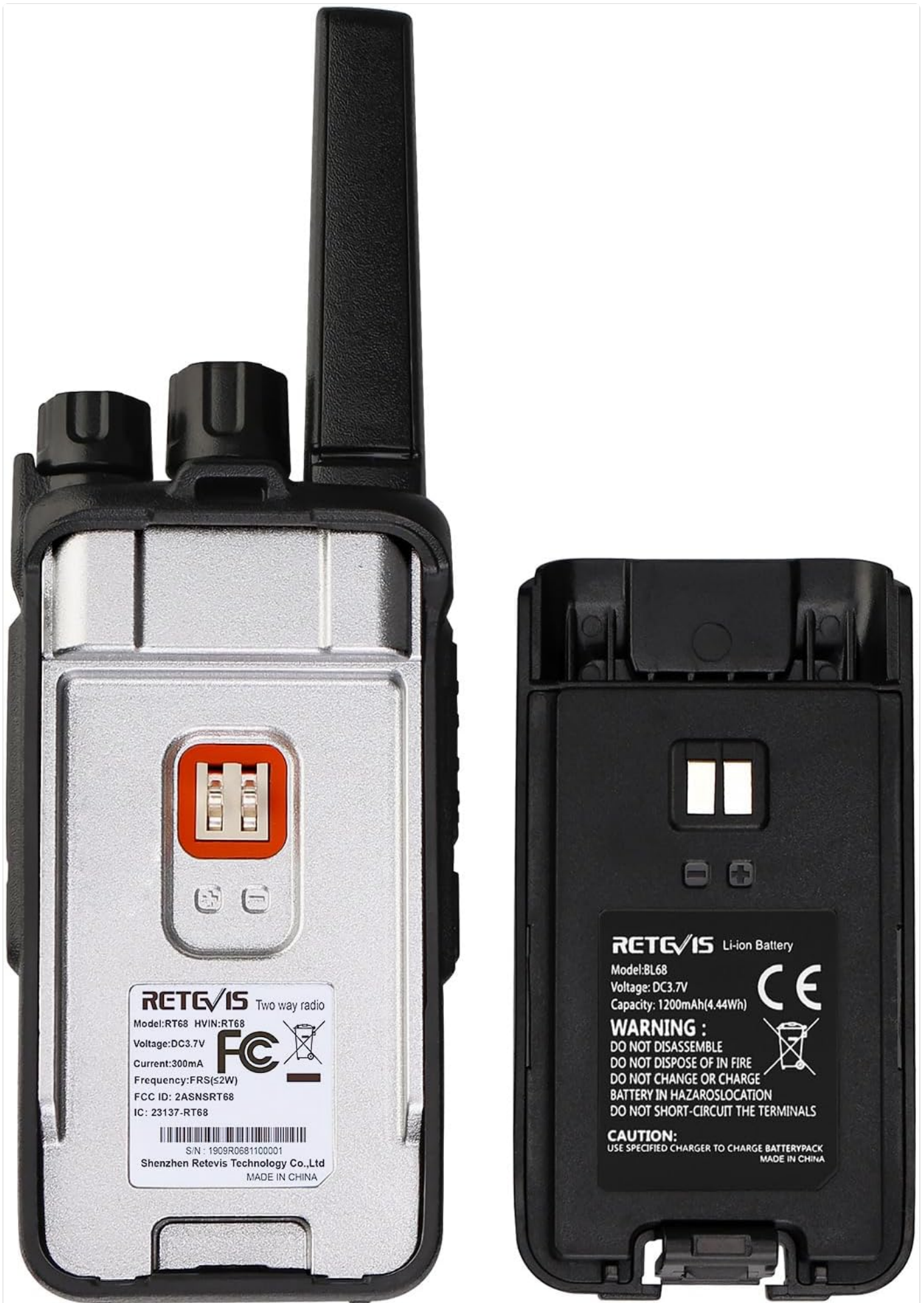
Figure 3: Battery compartment and battery pack.
