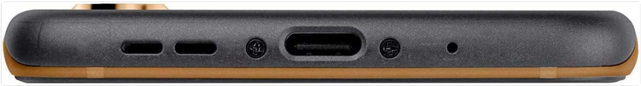
Image: Close-up of the Doro 8080's bottom edge, showing the USB-C charging port and other openings.
