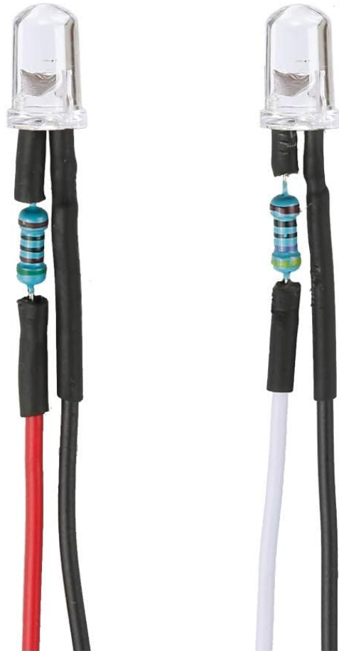
Figure 3.3: Detail of the preloaded 0.25W metal film resistor, ensuring stable operation at 12V.
