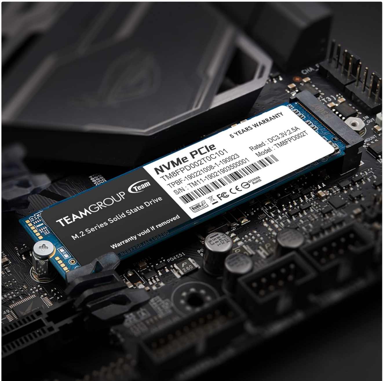
Figure 2: TEAMGROUP MP33 SSD installed in an M.2 slot on a motherboard.
