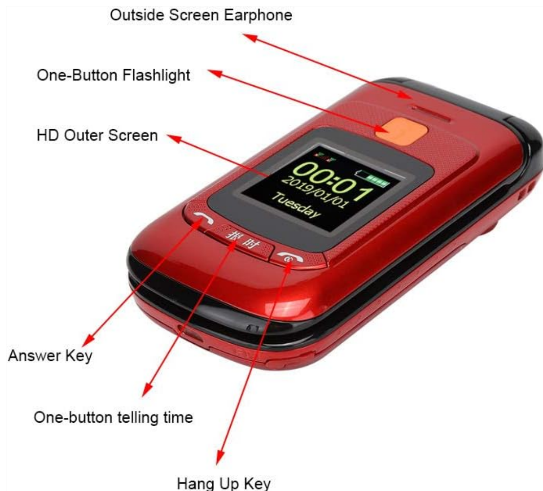
Image Description: A red ASHATA F899 flip phone shown from the front, closed. Labels point to the outside screen earpiece, one-button flashlight, HD outer screen, answer key, one-button telling time key, and hang up key.
