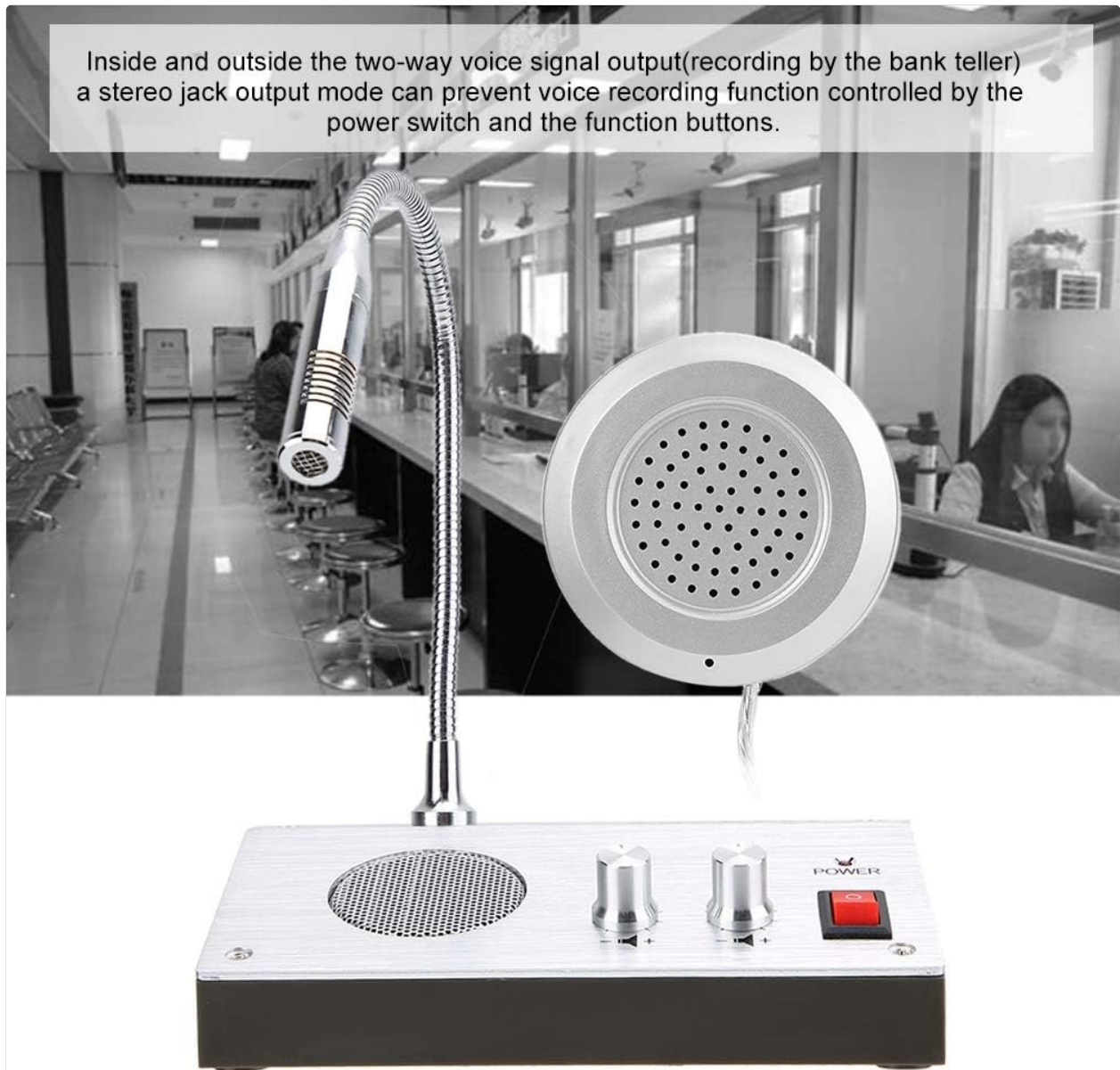
Figure 4.1: Illustration of the two-way voice output and recording capability.
