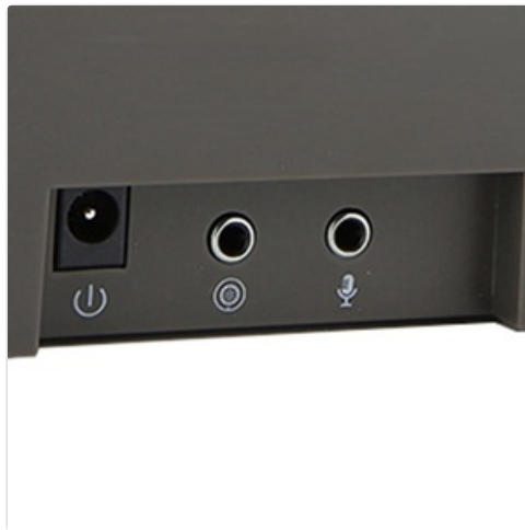
Figure 2.3: Rear ports for power, recording, and microphone/speaker connections.
