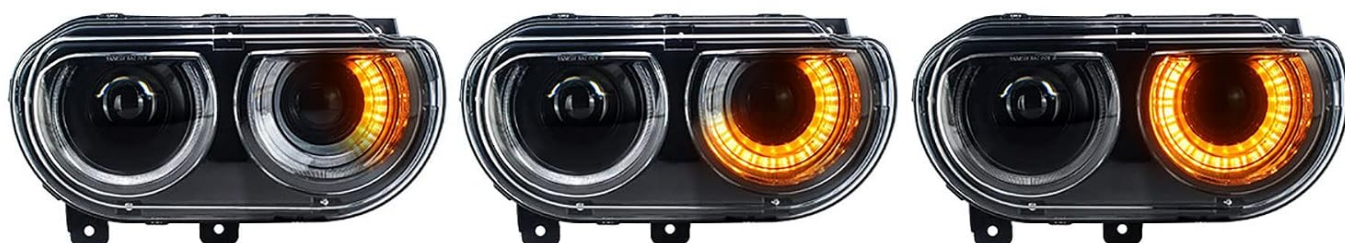
Image: Depiction of the sequential turn signal in action, showing the amber light flowing across the halo.
