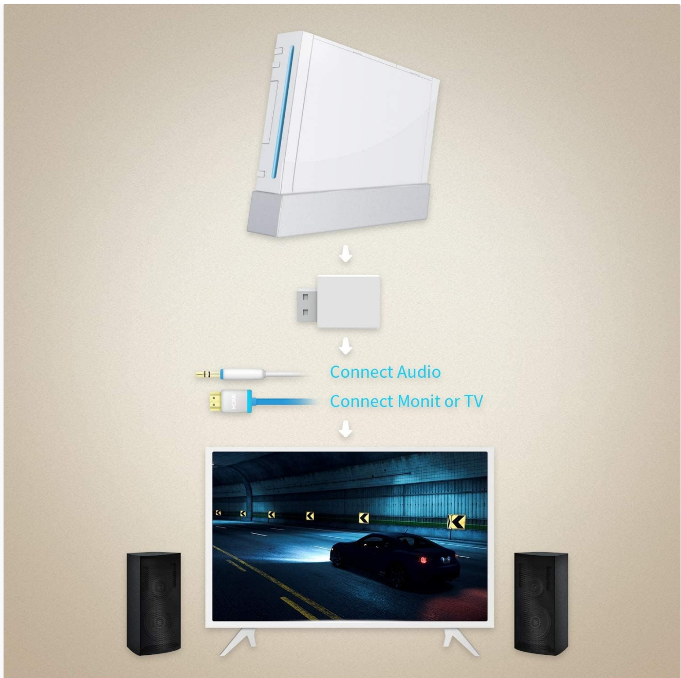
Image: A diagram illustrating the connection process: Wii console connects to the MAYFLASH converter, which then connects via HDMI to a TV/monitor and optionally via a 3.5mm audio jack to speakers.
