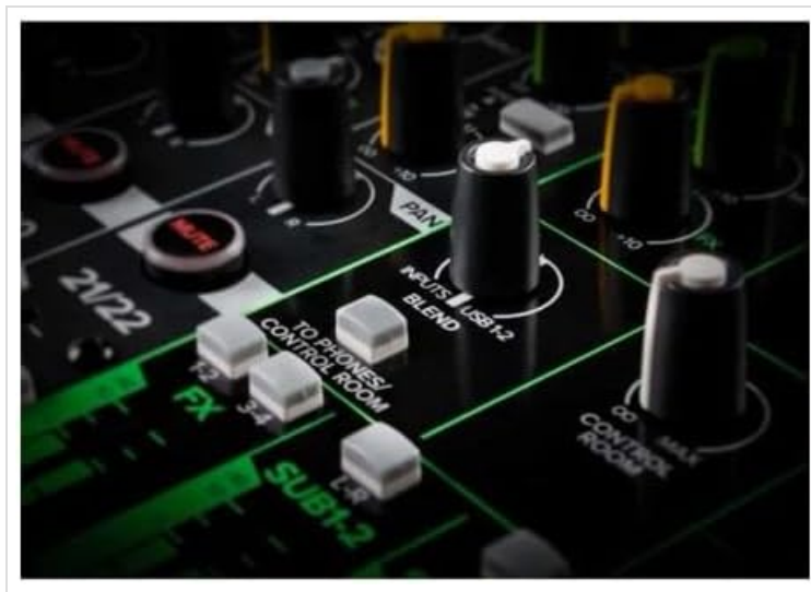
Image: A close-up view of the USB 1-2 Blend knob, which allows users to mix between the computer's output and the mixer's direct feed for monitoring.
