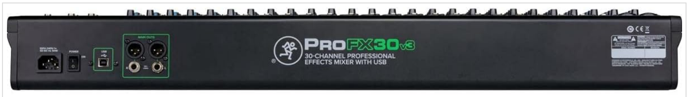
Image: The rear panel of the Mackie ProFX30v3 mixer, highlighting the power input, USB port, and main output connections.
