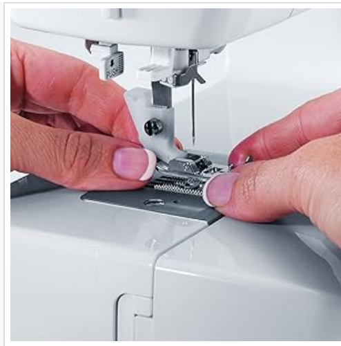
Figure 5: Demonstrating the adjustment of the presser foot for different fabric thicknesses.
