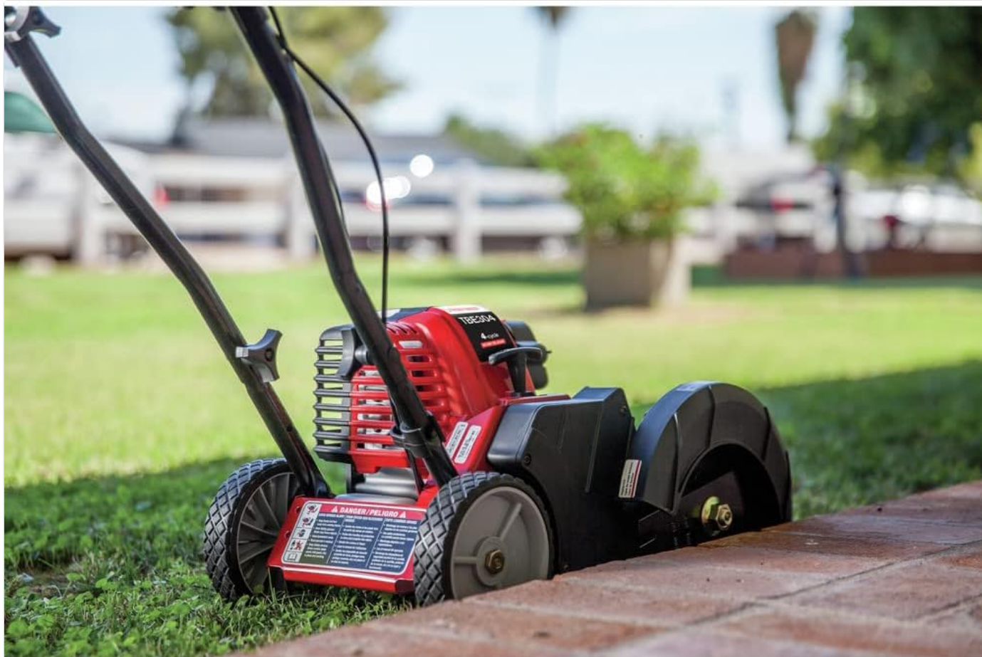
Figure 4: The edger in action, demonstrating its ability to create a precise and clean edge between a lawn and a paved surface.
