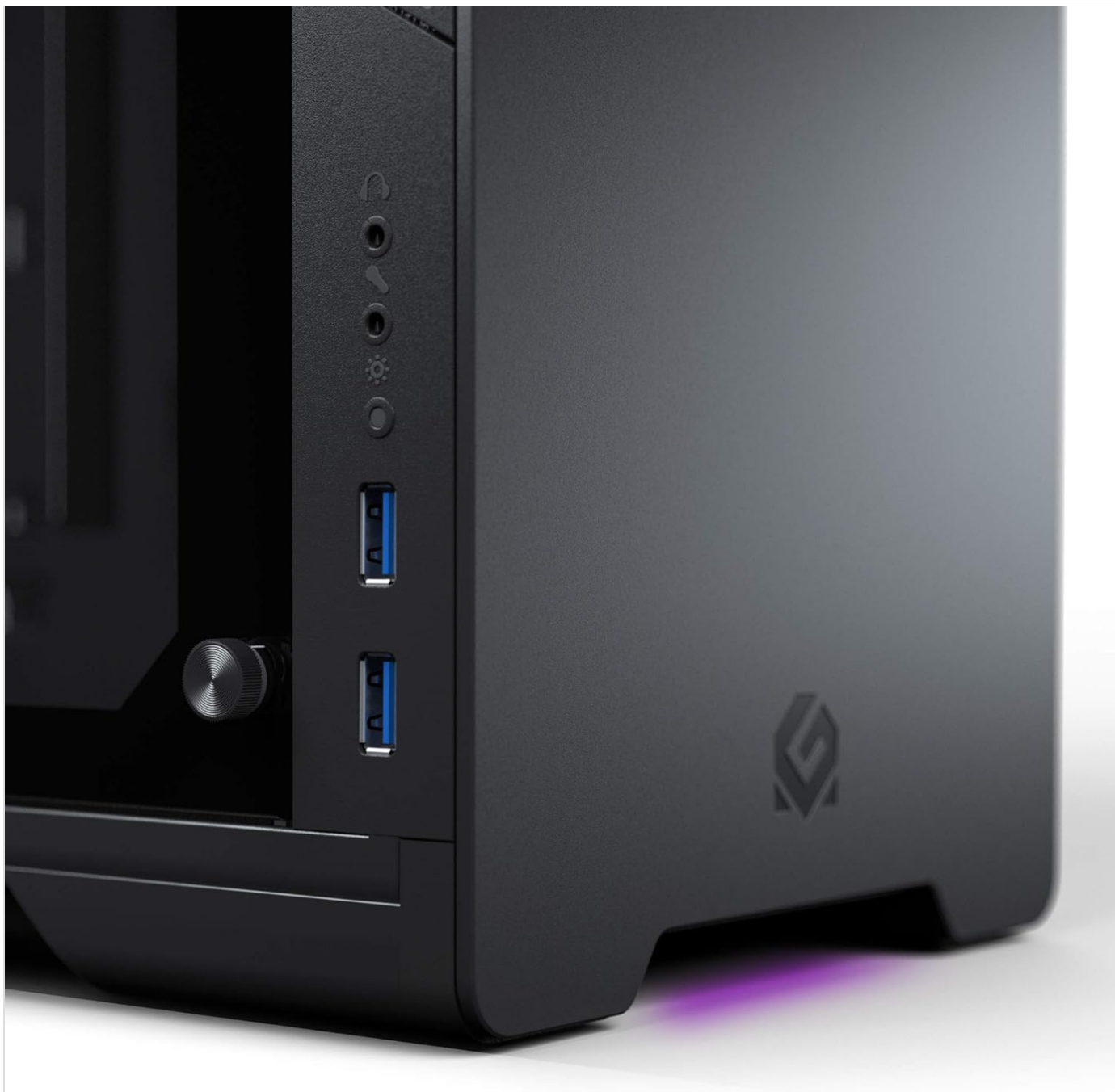
Figure 6: Front I/O panel showing USB 3.0 ports, audio jacks, and the RGB control button for quick connectivity and lighting adjustments.
