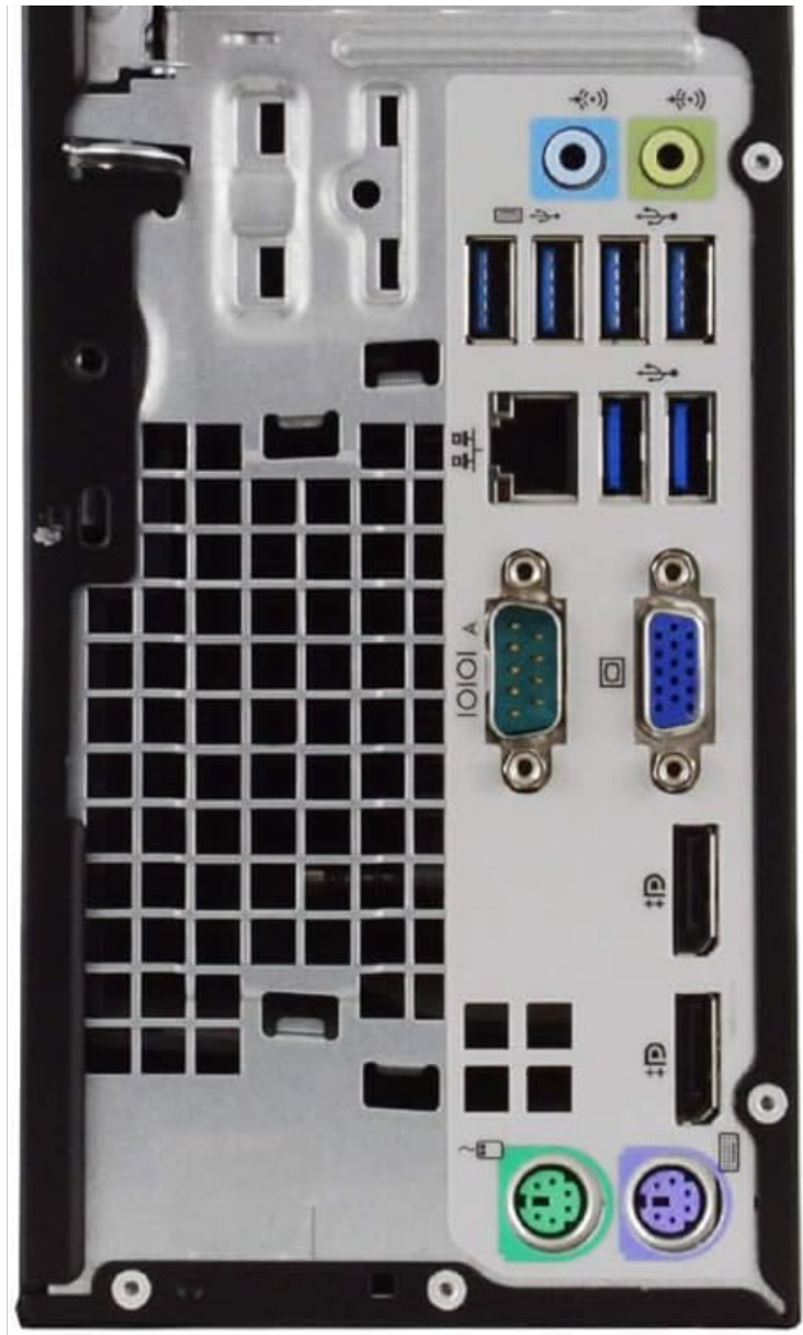
Image 4.1: Rear view of the HP EliteDesk 800 G2, illustrating the available ports for peripheral connections.
