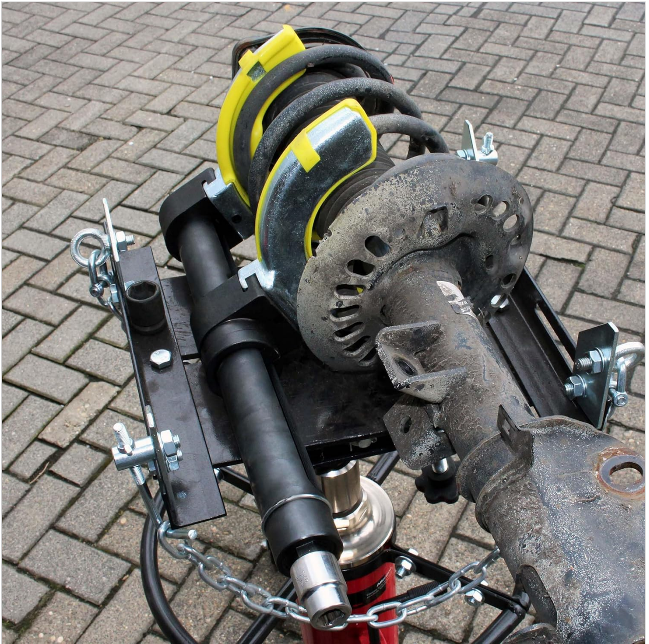
Image: A side view of the spring compressor engaged with a strut assembly, illustrating the tool's position and how it holds the spring under compression.
