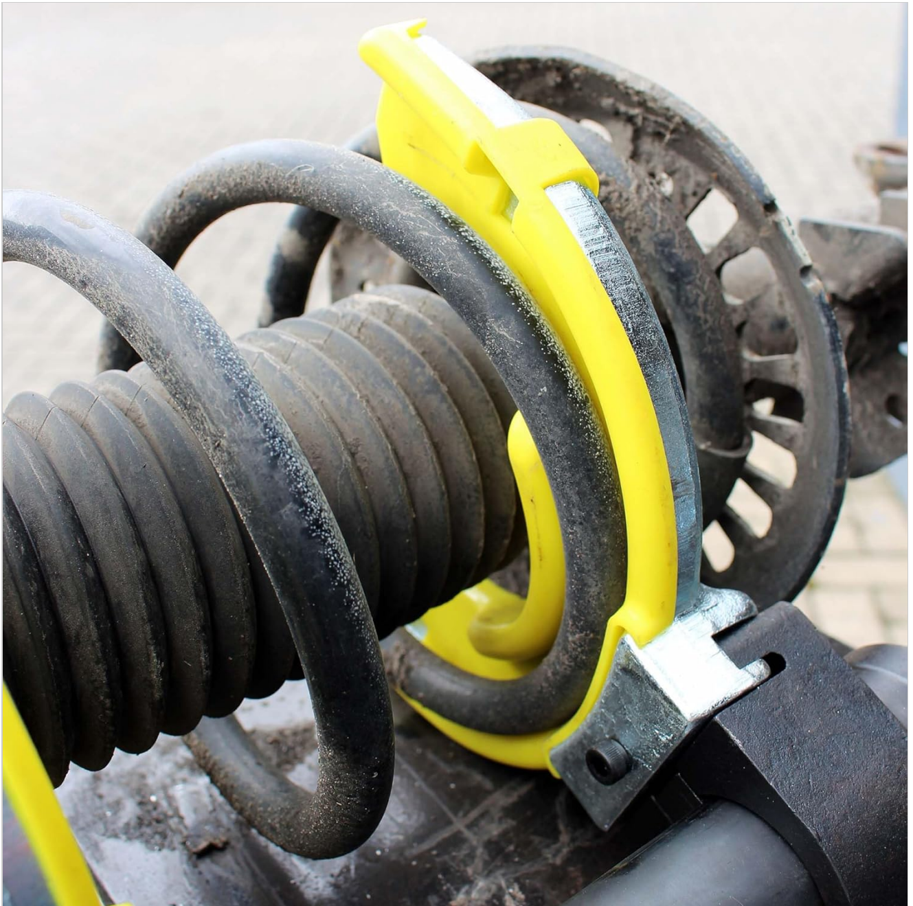
Image: A close-up of the yellow jaw clamps firmly gripping the coils of a vehicle spring, illustrating proper engagement before compression.
