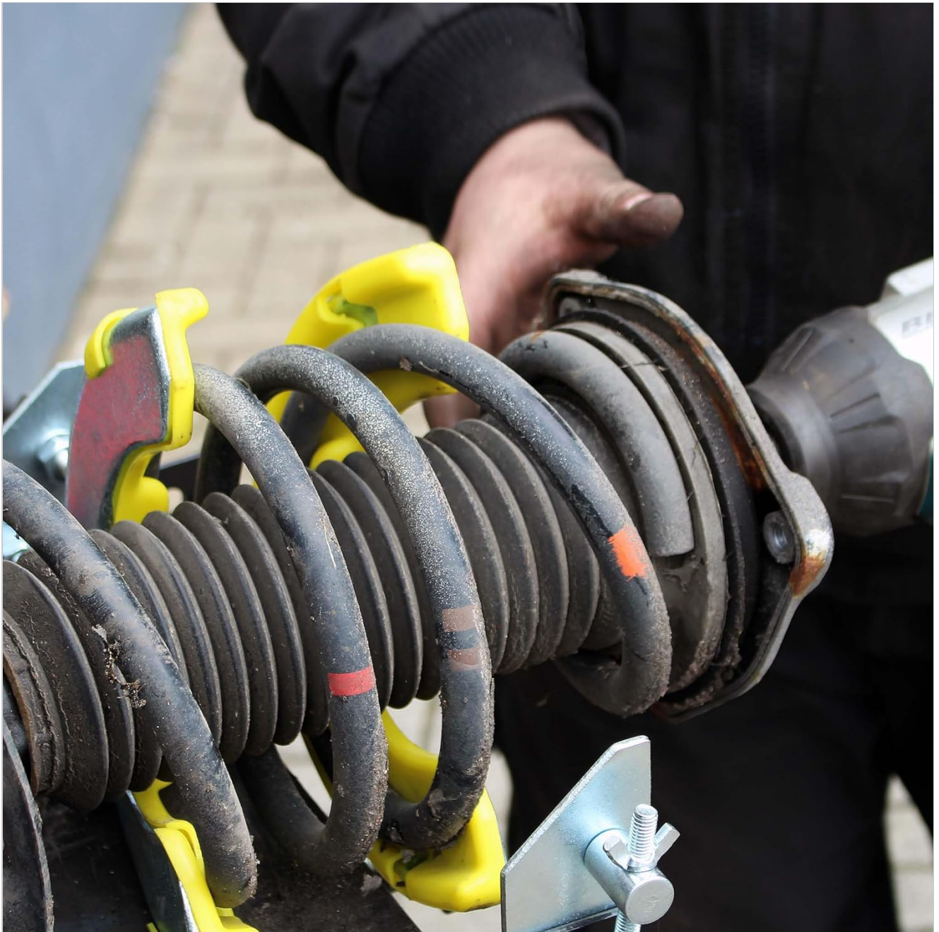
Image: A close-up of a gloved hand operating the spring compressor, demonstrating the manual adjustment process to compress or release the spring.
