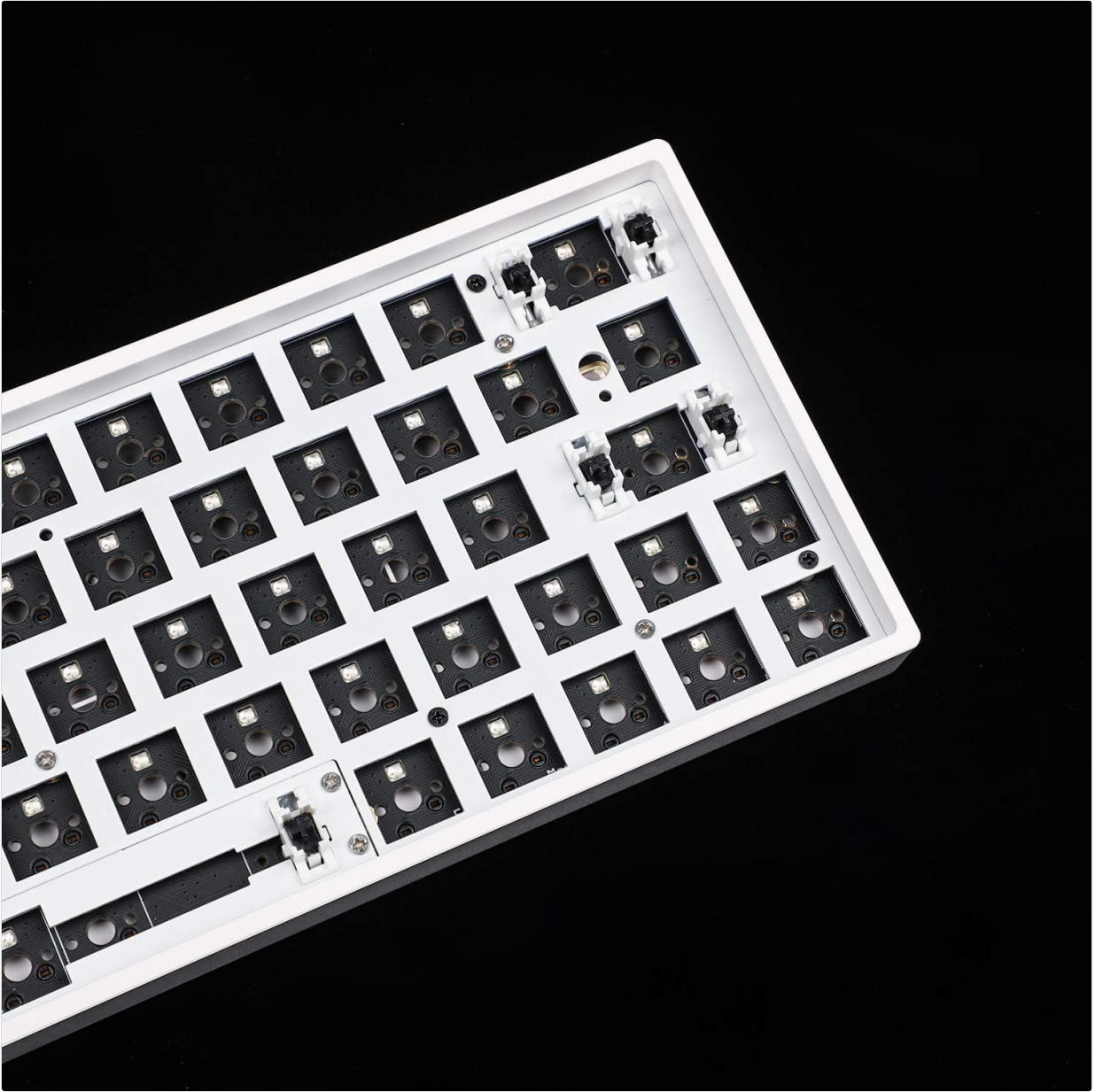
Figure 2: Angled view showcasing the plate and stabilizer mounts.
