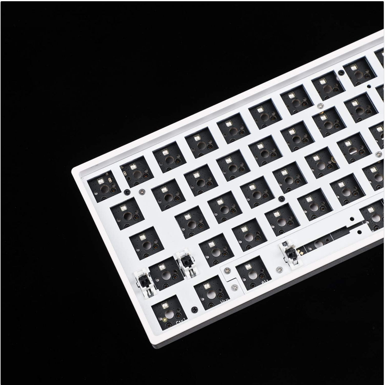
Figure 1: Top view of the assembled case and plate, ready for switches.
