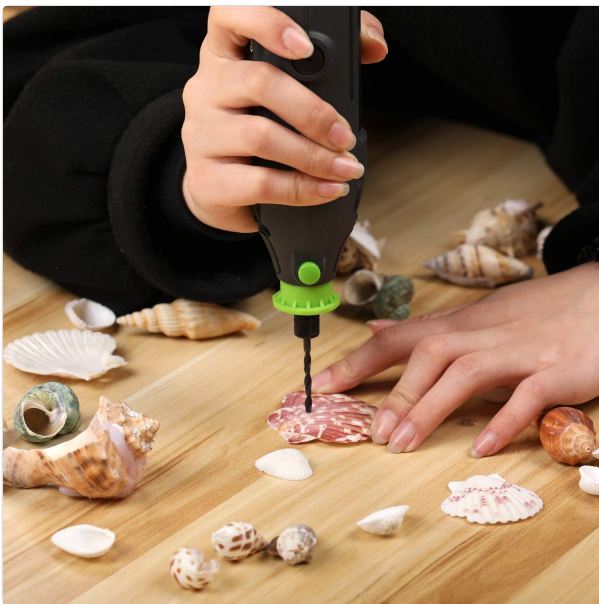
Figure 4.4: Drilling a seashell. Use appropriate drill bits and a controlled speed to prevent cracking.
