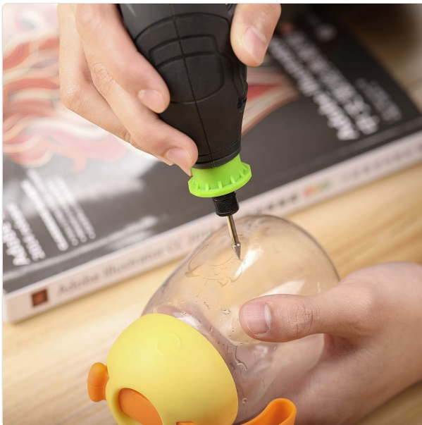
Figure 4.2: Engraving on glass. Use diamond bits and a lower speed for precise detailing.
