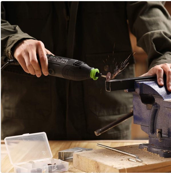
Figure 4.3: Cutting metal. Use cutting wheels and a higher speed, ensuring the workpiece is securely clamped.
