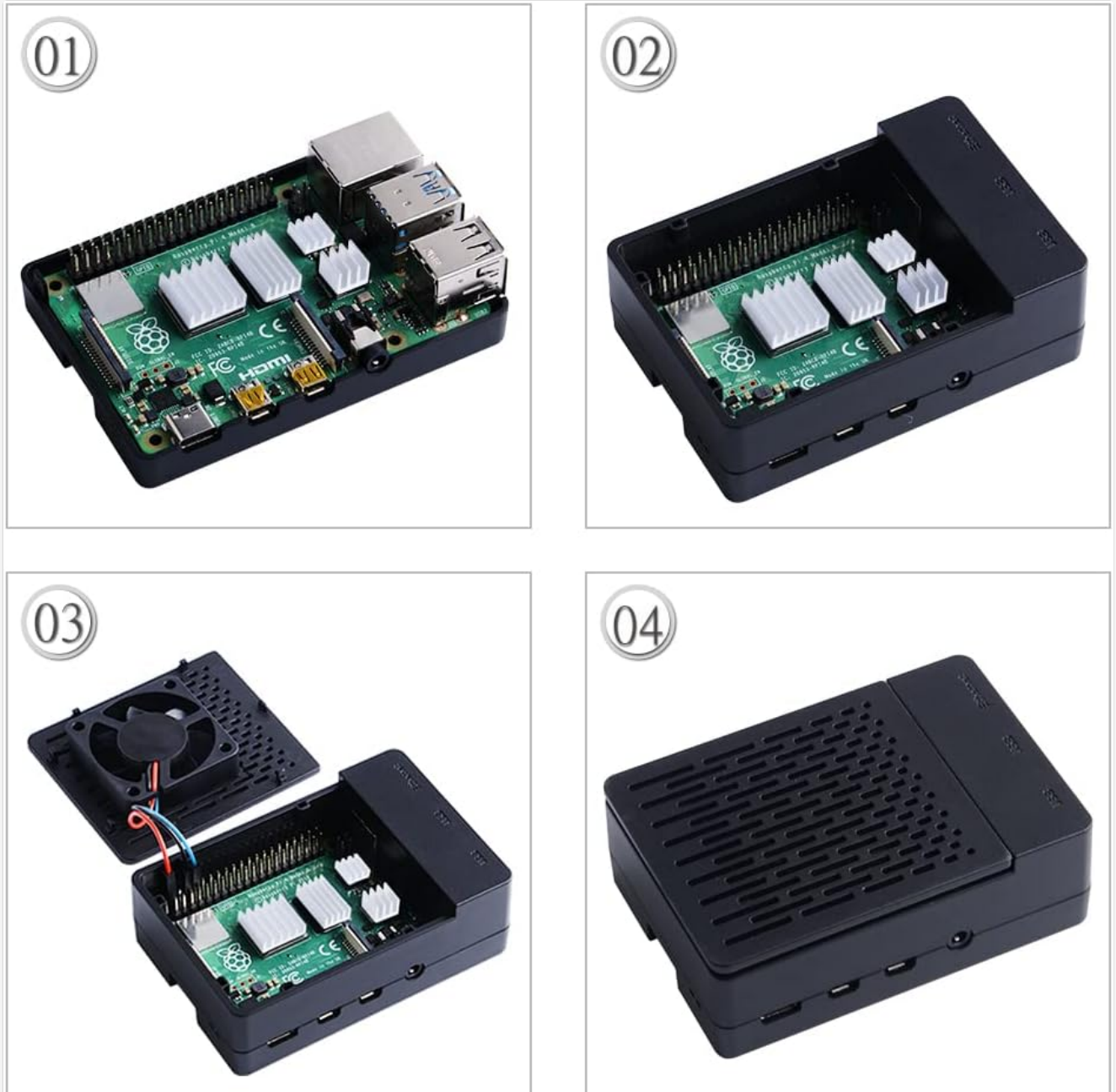
Figure 4: Step-by-step assembly process. This image illustrates the sequence of placing the Raspberry Pi into the case and attaching the fan and top cover.
