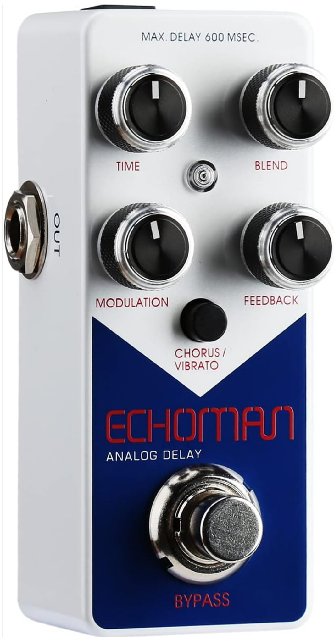
Image: Overview of the Xvive V21 Echoman pedal's controls.
