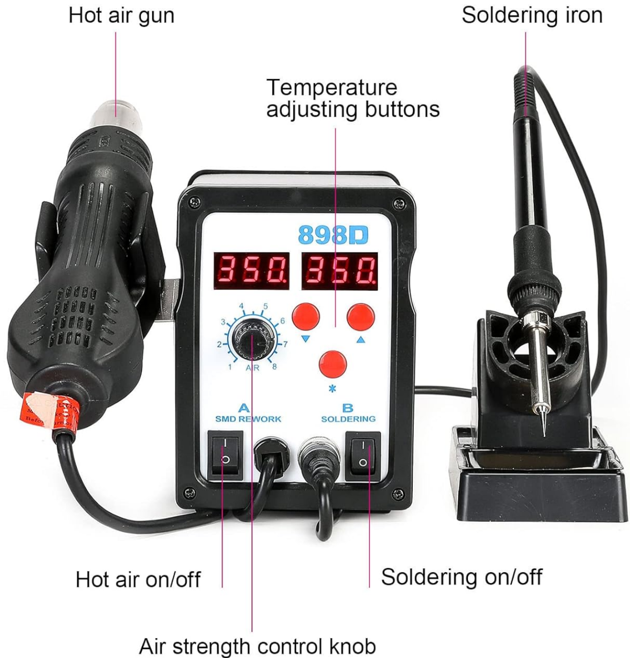
Figure 3: Labeled diagram of the rework station's main components and controls.
