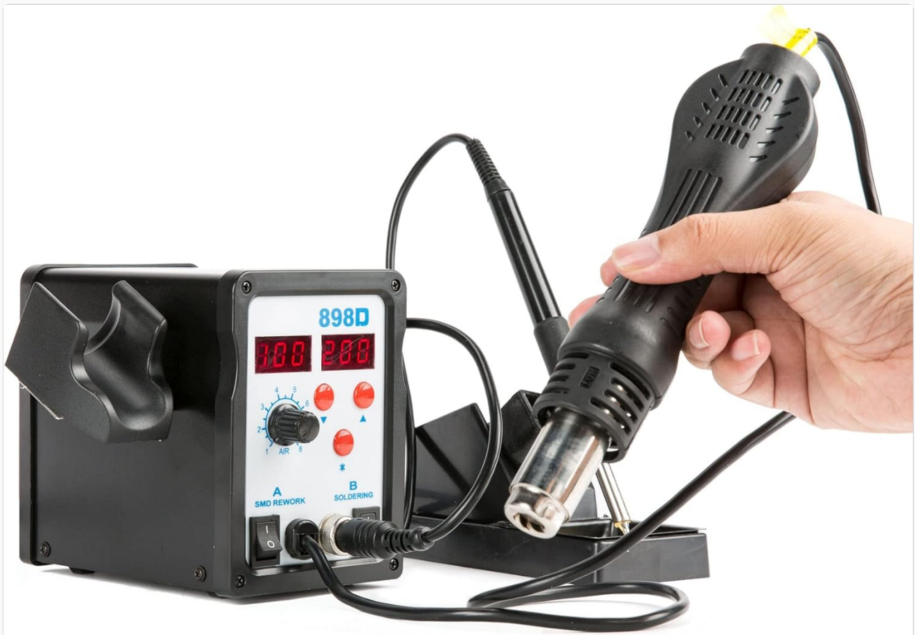
Figure 5a: Using the hot air gun for rework tasks.
