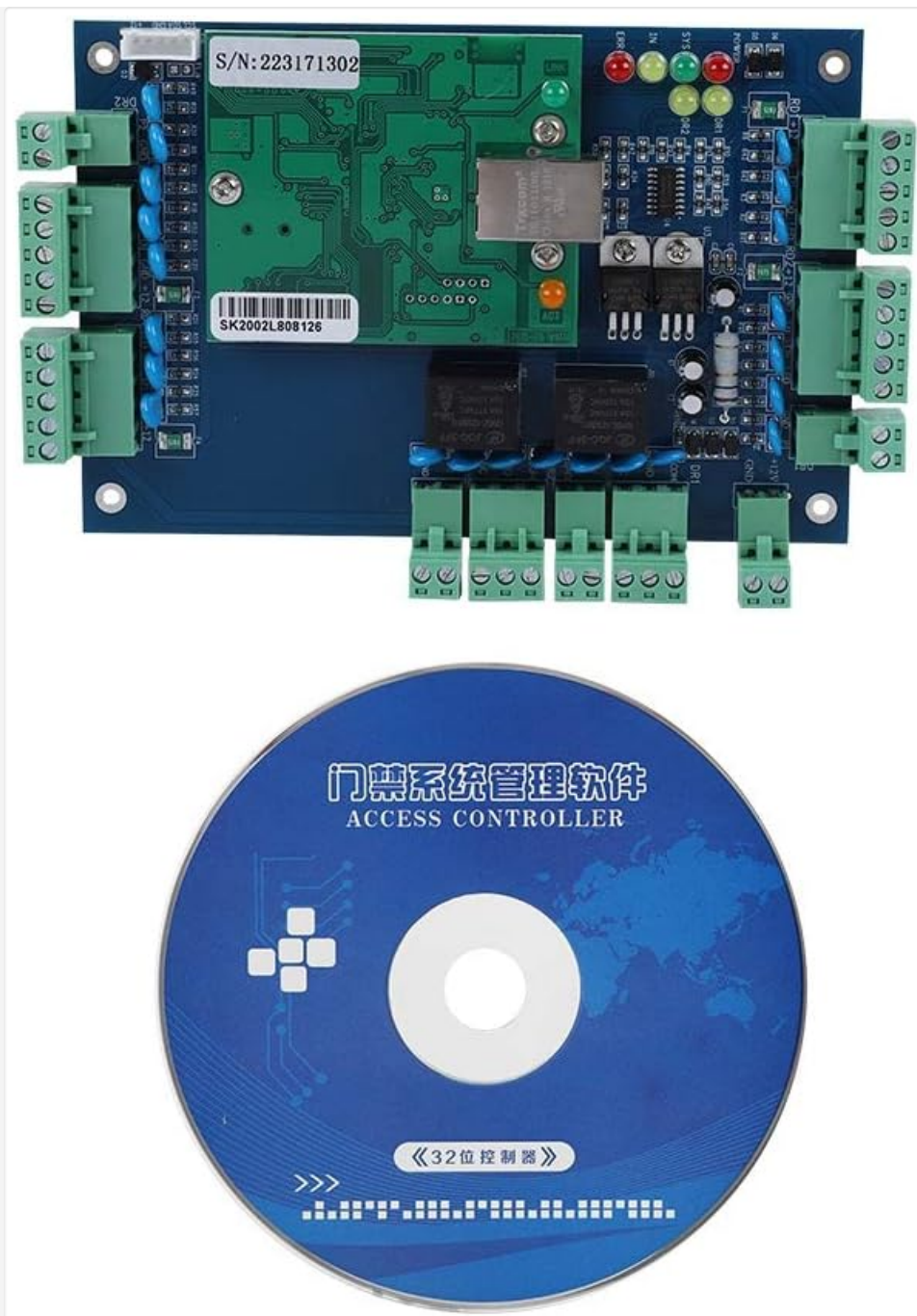
Image 3.1: The Wendry TCP/IP Network 2-Door Access Control Board and the accompanying software CD. The board features multiple connection terminals and an Ethernet port for network communication.
