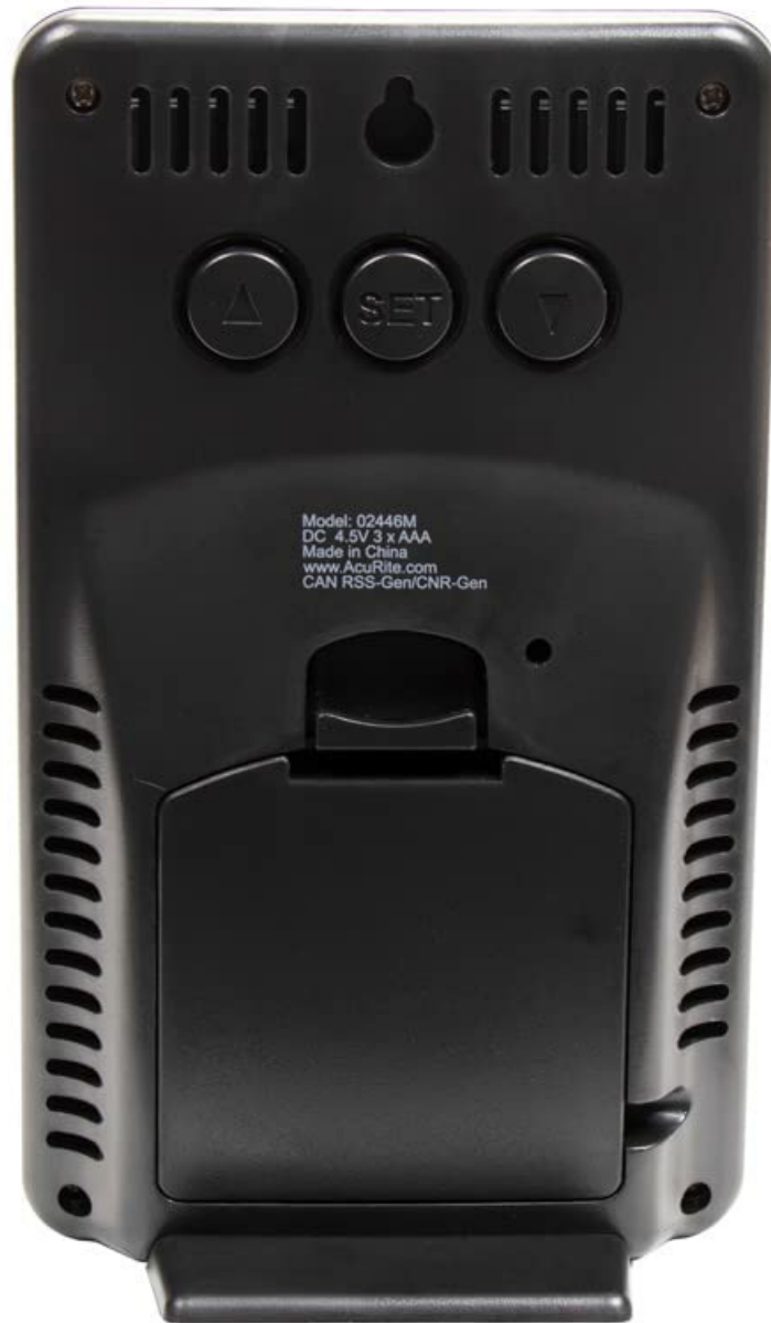
Figure 3.1: Back of the digital display unit, showing the battery compartment.
